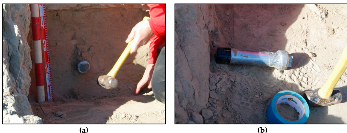
Figure 8. OSL sampling of CCMS-OSL-01: (a) Illustrates the sample tube being driven into the target sediments; (b) Shows the sample tube after retrieval and capping.
