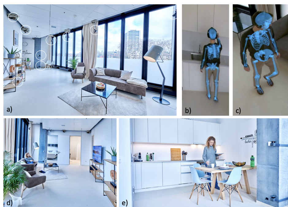
Figure 2. Marker-free motion tracking in the sensor-equipped apartment (NeuroTec Loft) University Hospital Inselspital. The living room (a,d) and the kitchen (e) are equipped with 13 cameras that allow to fit a 54-point skeleton model onto the test-person’s body (b,c).
