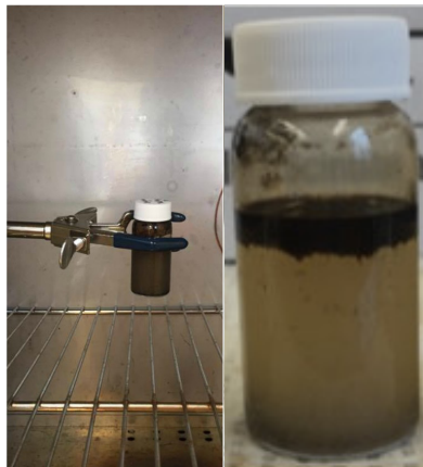
Figure 7. Left: Vial containing 1 g of SBos oil sand ( 10 \pm 1\% bitumen content), 15 mg SNP-g-PMEO 2 MA (15%, DS 0.022), 0.5 M NaCl, 60 mg toluene, and 15 mL water attached to a tumbler arm in an oven at 45 °C. Right: Bitumen floating to the surface 24 h after the extraction.
