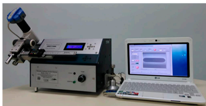
Figure 2. Oscillating spinning drop interfacial rheometer recent version.
