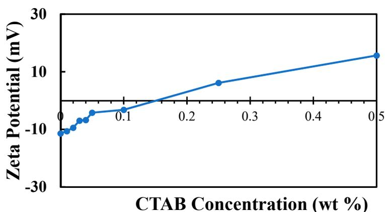
**Figure 6.** Variation of zeta potential and 1 wt% nanoclay dispersions as a function of CTAB concentration.
