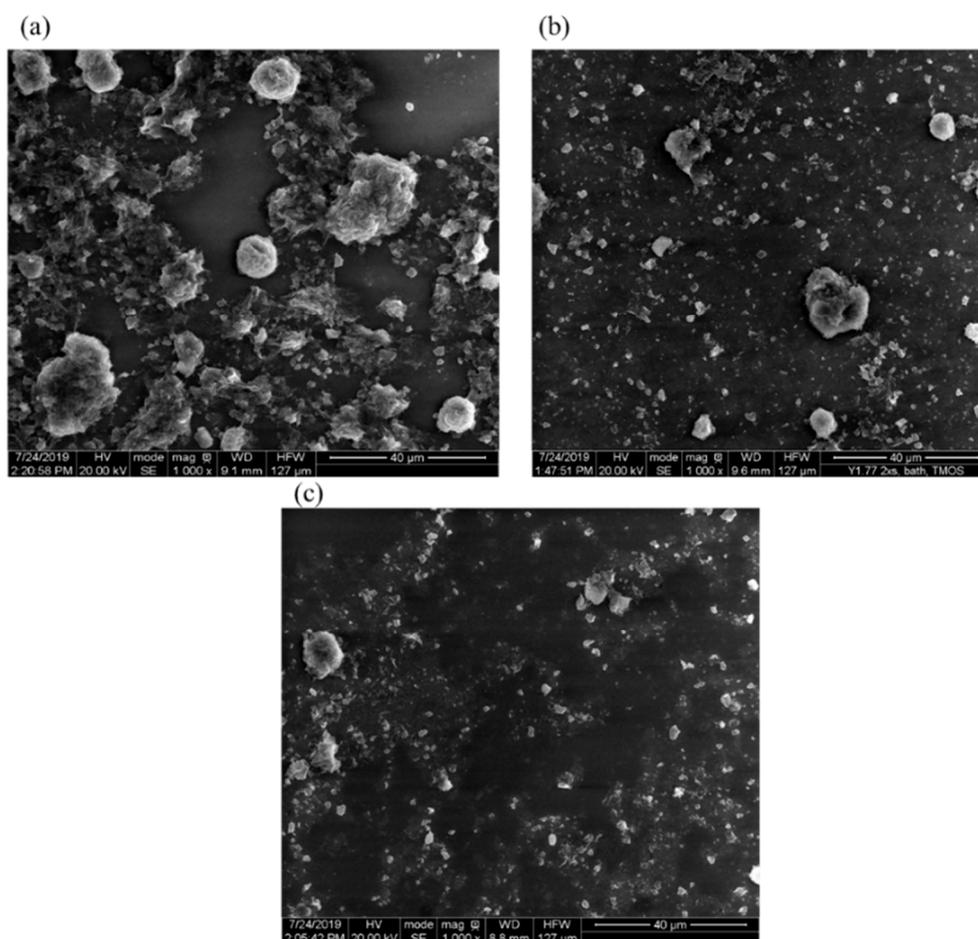
**Figure 4.** Scanning electron microscopy (SEM) images of dried 1 wt% aqueous dispersions of bentonite nanoclay (NC-Bt) in the presence of (a) 0 wt%, (b) 0.05 wt%, and (c) 0.1 wt% CTAB. Scale bar = 40 μm.
