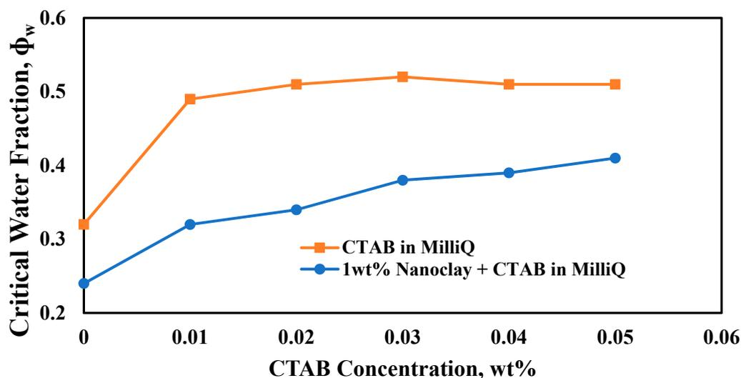
**Figure 16.** Comparison between plots of critical volume fraction of water versus varying CTAB concentrations for pure CTAB and 1 wt% nanoclay –CTAB mixture, respectively.
