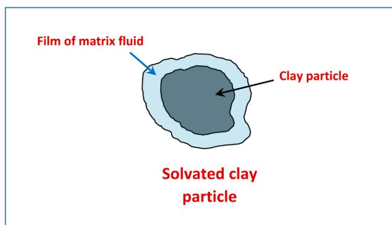
**Figure 3.** Nanoclay coated with immobilized dispersing aqueous film.
