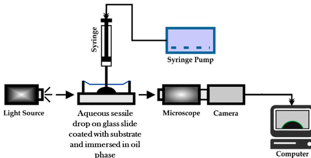
**Figure 2.** Schematic of the sessile drop method for measuring contact angle.
