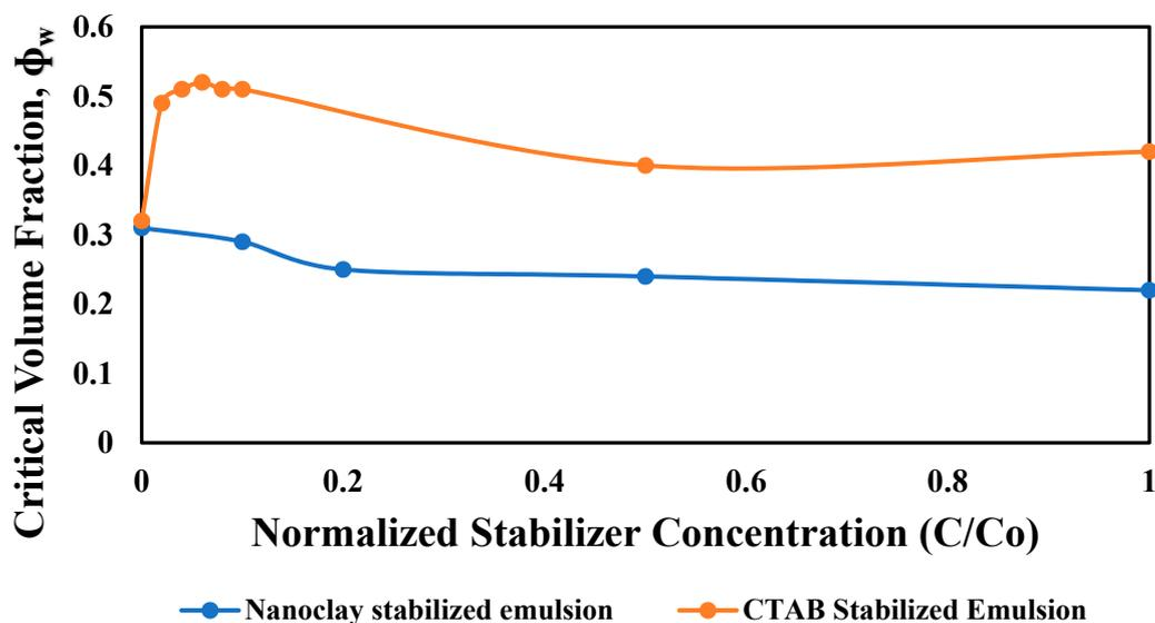
Figure 13. Aqueous phase critical volume fraction as a function of normalized concentration for CTAB and nanoclay.
