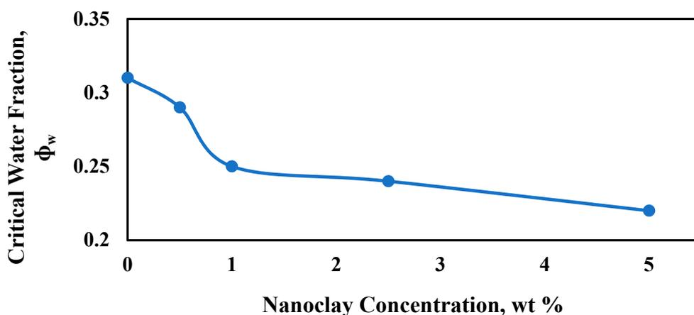
Figure 10. Critical volume fraction of water versus nanoclay concentration.
