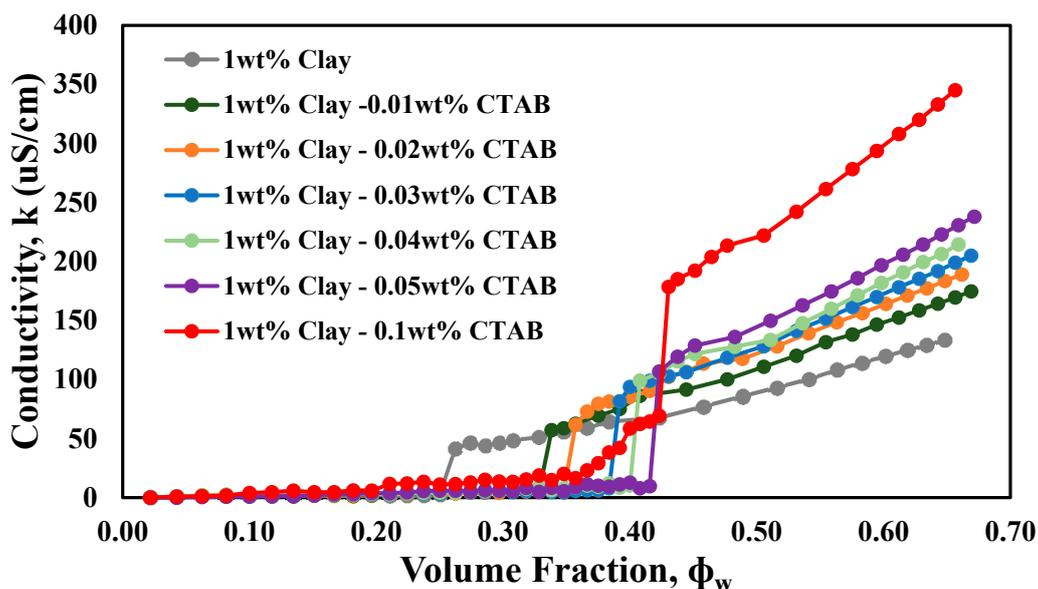
Figure 14. Conductivity of water–mineral oil emulsions stabilized by 1 wt% nanoclay at varying CTAB concentrations as a function of the volume fraction of water.
