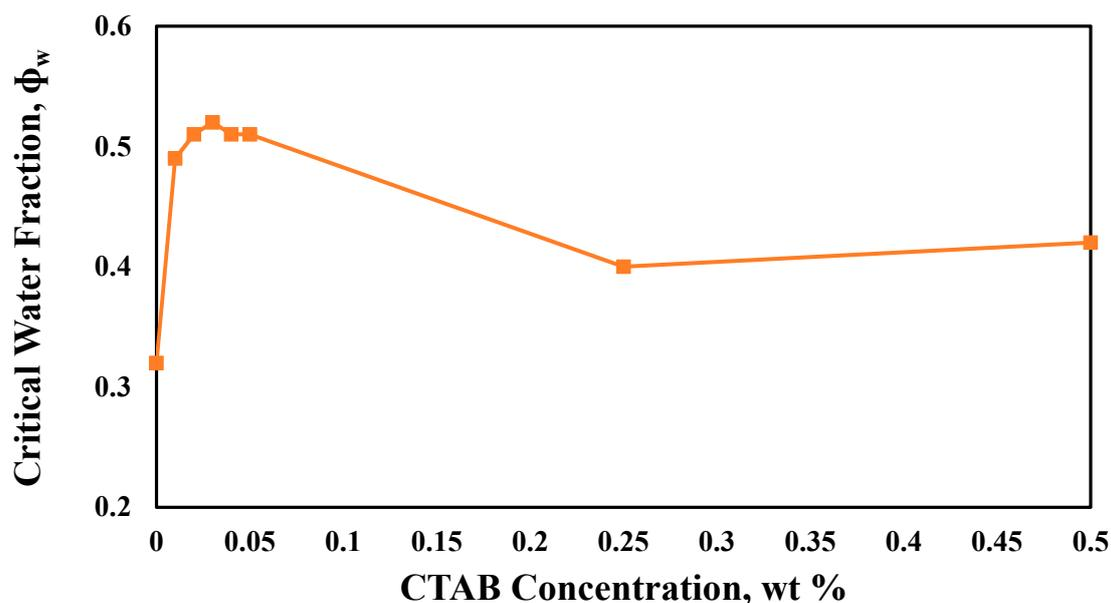
Figure 12. Critical volume fraction of water versus CTAB concentration.
