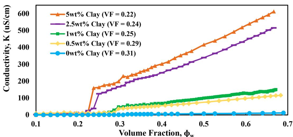
**Figure 9.** Conductivity of water–mineral oil emulsions stabilized by nanoclay solutions (0, 0.25, 0.5, 1, 1.75, 2.5, and 5 wt%) as a function of the volume fraction of water. Note: VF = volume fraction of water where phase inversion is observed.
