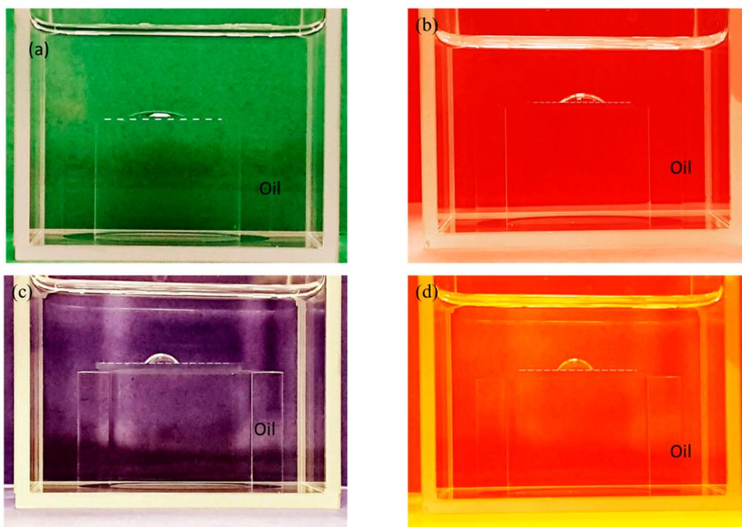
**Figure 8.** Images of sessile drop on glass slides coated with 1 wt% nanoclay with CTAB concentrations of: (a) 0, (b) 0.01, (c) 0.03, and (d) 0.05, immersed in the oil phase.
