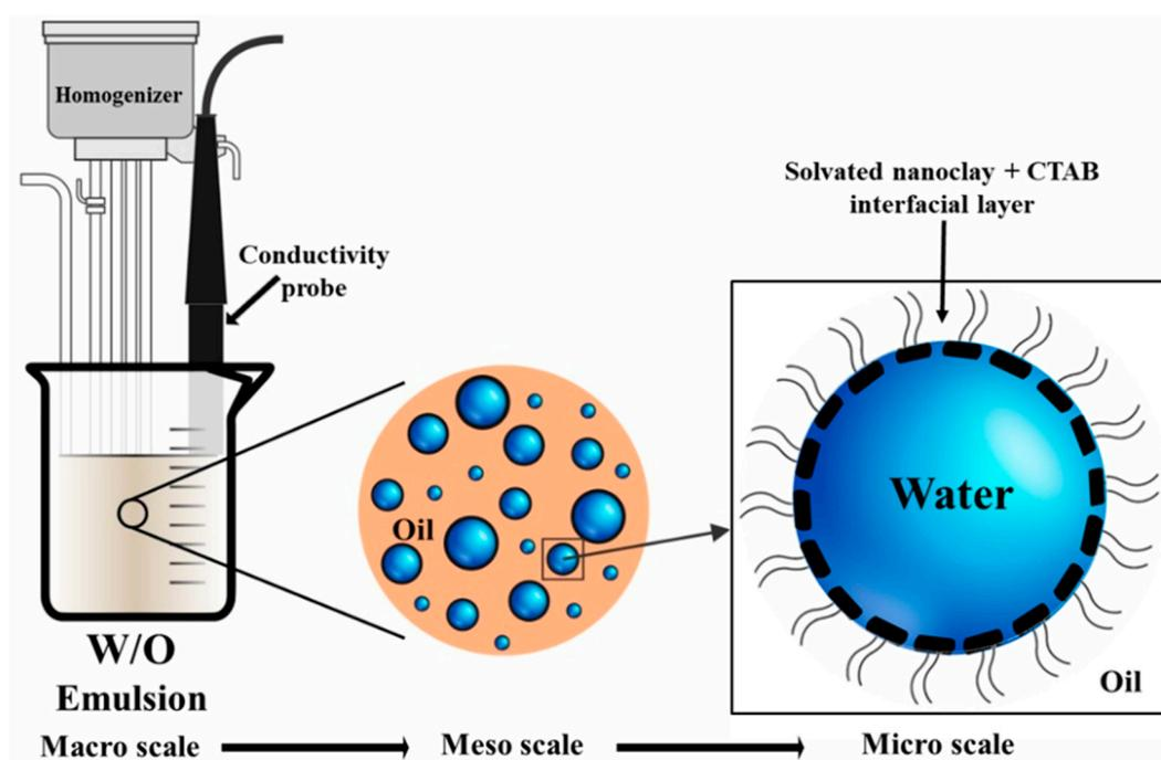
**Figure 1.** Schematic of a multiscale water-in-oil (W/O) emulsion system, with an emphasis on water droplets stabilized by surfactant-modified nanoclay. Note: CTAB = cetyltrimethyl ammonium bromide.
