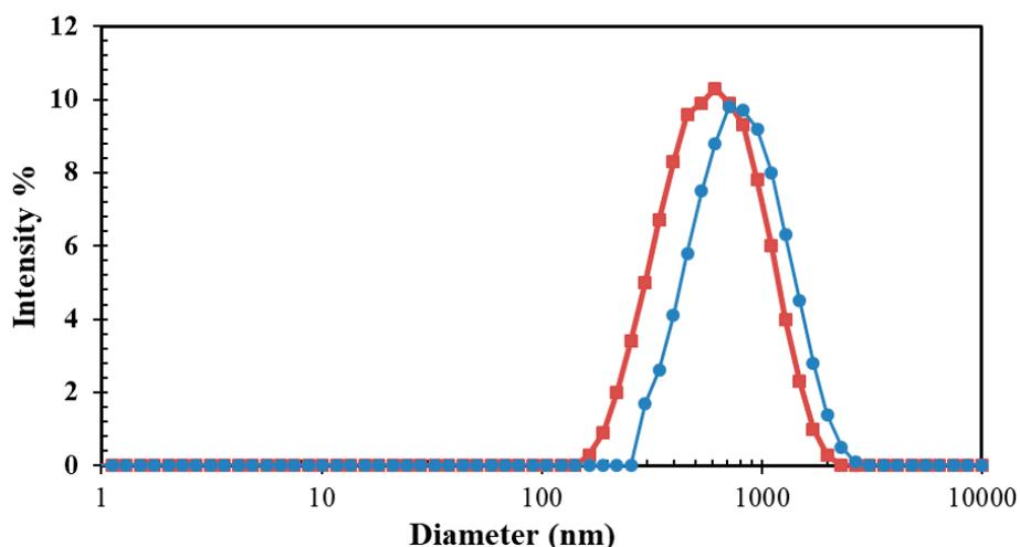
**Figure 5.** Particle size distribution of 0.1 wt% and 1 wt% nanoclay dispersions using DLS: 0.1 wt%, blue circle; 1 wt%, red square.
