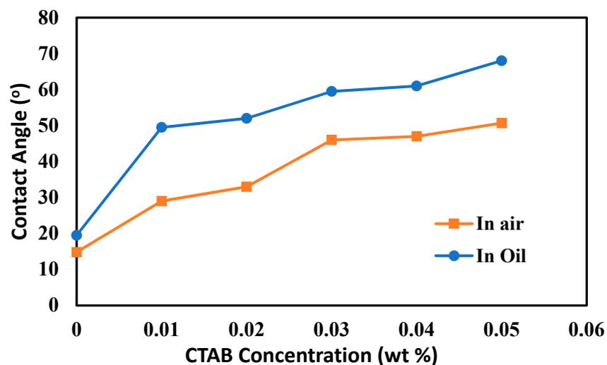
**Figure 7.** Variation of contact angles measured of a water drop in air (squares) and in oil (circles) as a function of CTAB concentration in a 1 wt% nanoclay dispersion.
