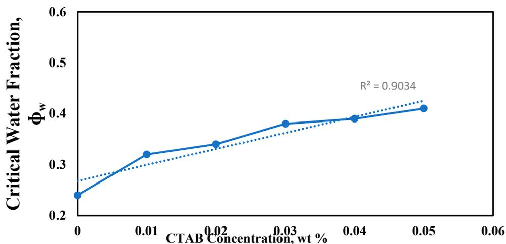
**Figure 15.** Critical volume fraction of water versus CTAB concentration in 1 wt% nanoclay–CTAB mixture.
