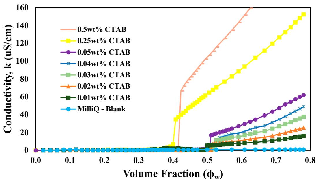
Figure 11. Conductivity of water-mineral oil emulsions stabilized by pure CTAB solutions (0, 0.01, 0.02, 0.03, 0.04, 0.05, 0.25, and 0.5 wt%) as a function of the volume fraction of water.
