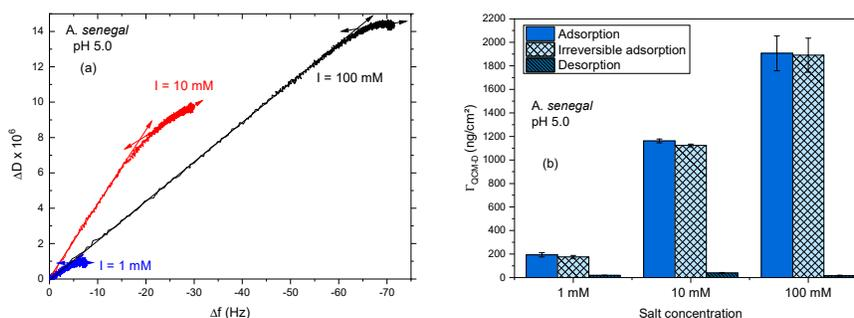
**Figure 5.** Adsorption of *A. senegal* gum at 150 ppm on gold substrate at pH 5.0 as a function of the salt concentration: (a)  $D$ - $f$  third normalized overtone profiles upon adsorption and (b) comparison of the adsorbed amount ( $\Gamma_{QCM-D}$ ) at equilibrium after adsorption and desorption (washed with buffer solution).
