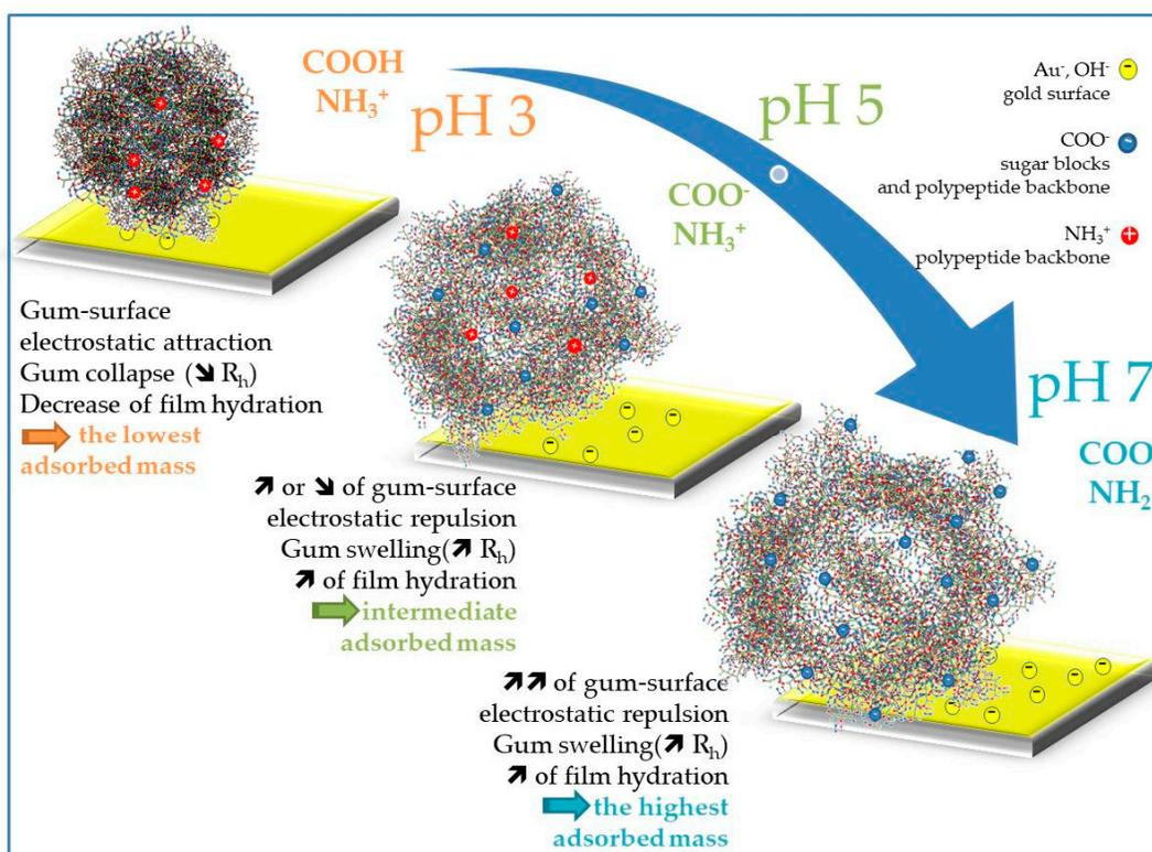
**Figure 10.** Scheme showing the electrostatic interactions and conformational changes as a function of the pH occurring when *A. senegal* gum adsorbed onto the gold substrate. Note that the hydrodynamic radii ( $R_h$ ) changes as a function of the pH were experimentally demonstrated (data not shown).
