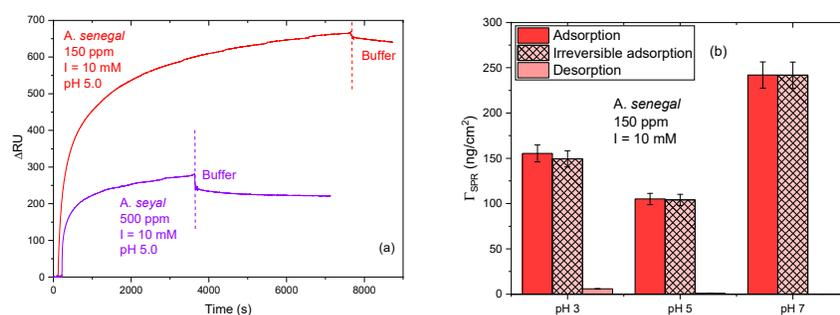
**Figure 4.** (a) Surface Plasmon Resonance SPR sensorgram illustrating the immobilization of *A. senegal* and *A. seyal* gums at pH 5.0 and 10 mM acetate buffer on gold substrate. (b) Comparison of the adsorbed amount ( $\Gamma_{SPR}$ ) of *A. senegal* gum on the gold substrate at equilibrium after adsorption and desorption (washed with buffer solution) at pH 3.0, 5.0, and 7.0.
