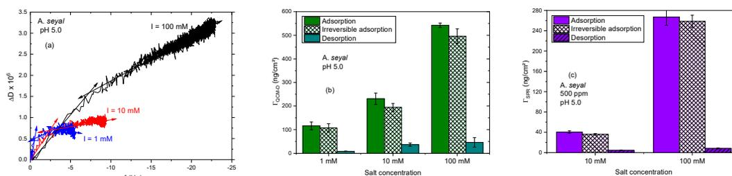
**Figure 7.** Adsorption of *A. seyal* gum at 500 ppm on gold at pH 5.0 as a function of the salt concentration: (a)  $D$ - $f$  third normalized overtone profiles upon adsorption and (b) comparison of the adsorbed amount,  $\Gamma_{QCM-D}$  (ng/cm<sup>2</sup>) and (c)  $\Gamma_{SPR}$  (ng/cm<sup>2</sup>), of *A. seyal* gum on the gold substrate at equilibrium after adsorption and desorption (washed with the buffer solution).
