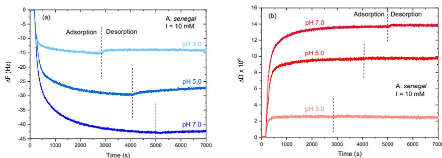
**Figure 2.** Adsorption kinetics of *A. senegal* gum at 150 ppm in 10 mM acetate buffer on gold substrate as a function of pH: (a) frequency change ( $\Delta F$ ) and (b) dissipation energy loss ( $\Delta D$ ). Dashed lines represent the switch of the solution from the adsorption to desorption process with acetate buffer.
