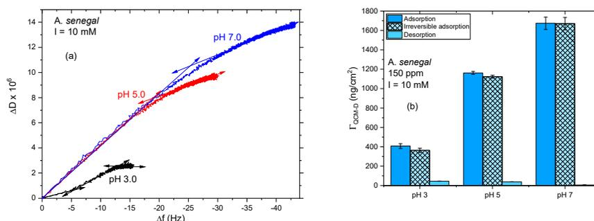
**Figure 3.** Adsorption of *A. senegal* gum at 150 ppm in 10 mM acetate buffer on gold substrate as a function of the pH: (a)  $D$ - $f$  third normalized overtone profiles upon adsorption and (b) comparison of the adsorbed amount ( $\Gamma_{\text{QCM-D}}$ ) onto the gold substrate at equilibrium after adsorption and desorption.
