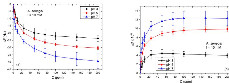
**Figure 1.** Adsorption isotherms of *A. senegal* gum on gold substrate presented as (a) frequency change ( $\Delta F$ ) and (b) dissipation energy loss ( $\Delta D$ ) for pH 3.0, 5.0, and 7.0 at a salt concentration of 10 mM acetate buffer. Time of adsorption between each concentration ranged from 30 to 60 min.
