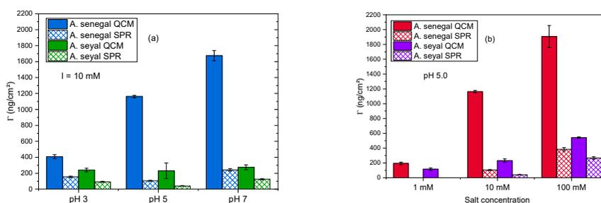
**Figure 9.** Comparison of the adsorbed mass amount of *A. senegal* and *A. seyal* gums on gold substrate obtained using QCM-D and SPR techniques: (a) as a function of the pH with a salt concentration of 10 mM acetate buffer and (b) as a function of the salt concentration with a constant pH 5.0.
