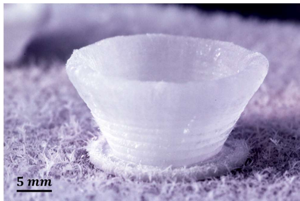
Figure 8. 3D DCW of 1:50 XG:CNC frozen vase with \approx 120^\circ angles, printed directly without using a support material.
