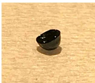
**Figure 5.** Photograph of an asphaltenes layer formed at the surface of the drop of decane/toluene (45/55 wt%) containing 5 wt% of asphaltenes at  $t = 2500$  s.
