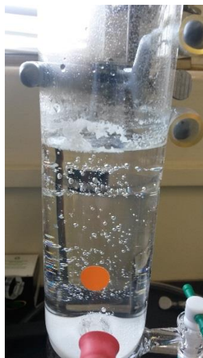
Figure 3. Scum concentrating on the solution surface and adsorbing to the column while floating \text{La}^{3+} at \varphi = 2 .
