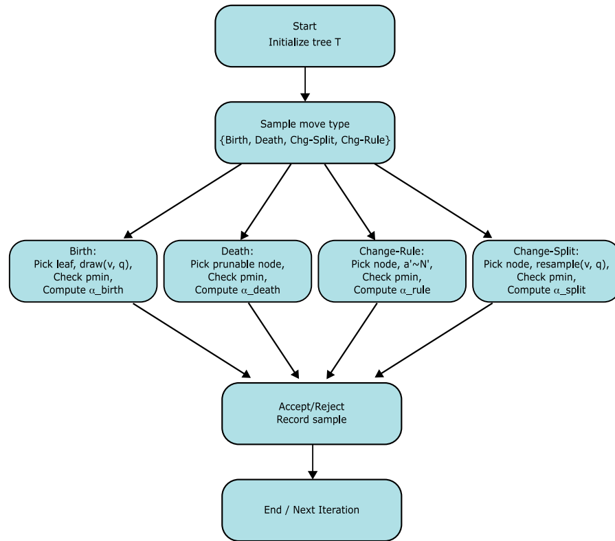
Figure 1. Flowchart of the RJ-MCMC sampler with birth, death, change-split, and change-rule moves. The sweeping strategy enforces the minimum leaf size p_{\min} by rejecting or collapsing unavailable proposals, ensuring reversibility and regularizing tree size.
