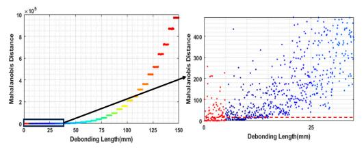
Figure 15. Estimated MSD values for debonding sizes of 10 mm to 150 mm located at 265 mm.
