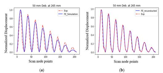
**Figure 14.** The first vibrational mode shape displacement data for scan points 1 to 208 (one-symmetric part): (**a**) original FE-simulated and experimental; (**b**) transformed FE-simulated and experimental data for debonding of 50 mm at 265 mm.
