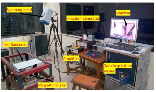
Figure 6. Experimental set-up of the LDV.
