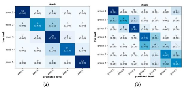
**Figure 17.** Confusion matrix for (**a**) debonding location zone and (**b**) debonding size group, as predicted by stacked model.
