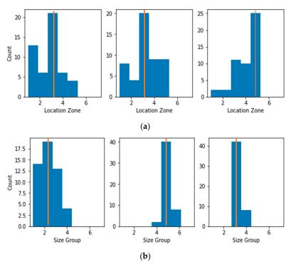
**Figure 19.** Results with experimental data, with stacked model trained with FE-transformed data with two-percent Gaussian noise for debonding (**a**) location zone and (**b**) size group; the histogram shows predicted labels, while the actual labels are marked by a yellow line.
