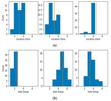
**Figure 18.** Results with experimental data, with stacked model trained with FE-transformed data without noise for debonding (**a**) location zone and (**b**) size group; the histogram shows predicted labels, while the actual labels are marked by a yellow line.
