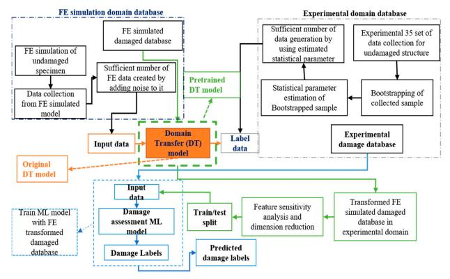
Figure 2. Domain-transfer-based SHM methodology framework.
