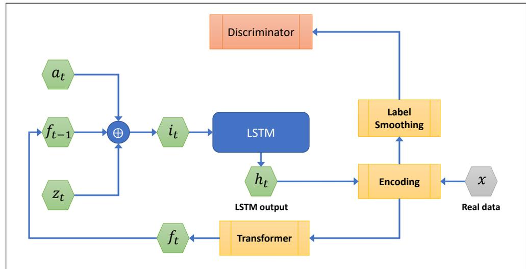
**Figure 11.** DATGAN process flow diagram.
