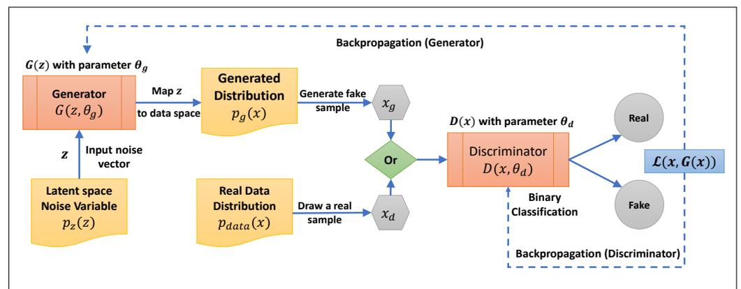
Figure 2. GAN process flow diagram.
