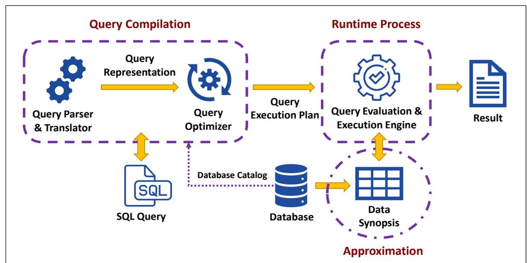
Figure 1. Query processing flow diagram in AQP.
