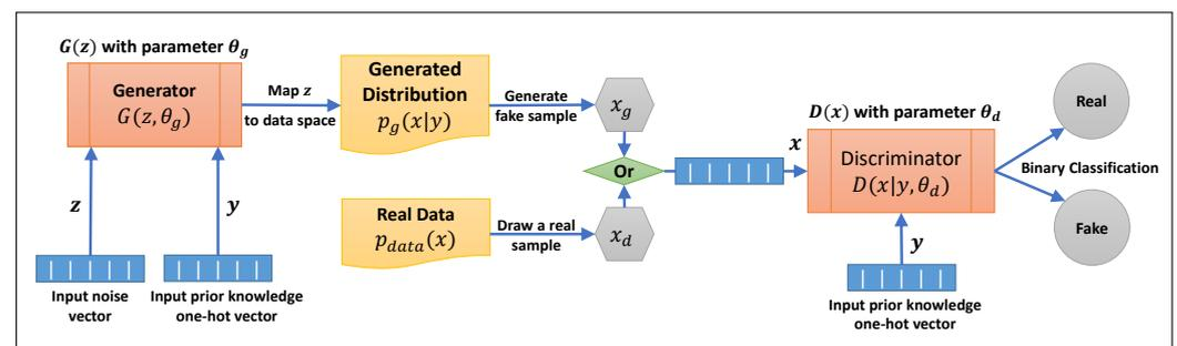
**Figure 3.** Conditional GAN process flow diagram.
