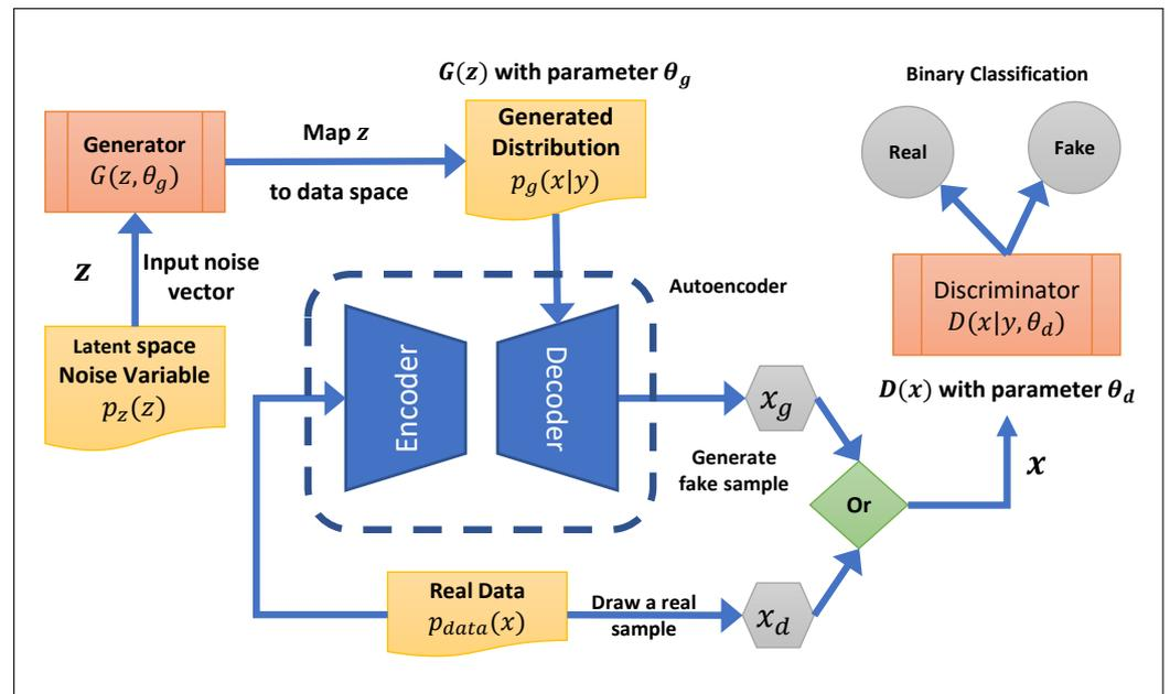
Figure 4. The medGAN architecture: the discriminator utilizes an autoencoder (which is trained by real data) to receive a decoded random noise variable.
