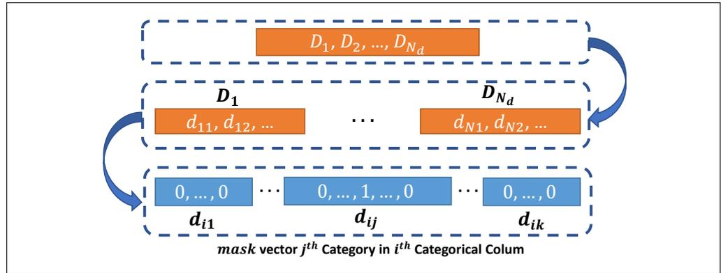
**Figure 10.** Following vectorization of categorical columns, all vectors are initialized with 0; then, the  $j^{th}$  category from the  $i^{th}$  column is selected and the value of the corresponding element is changed to 1.
