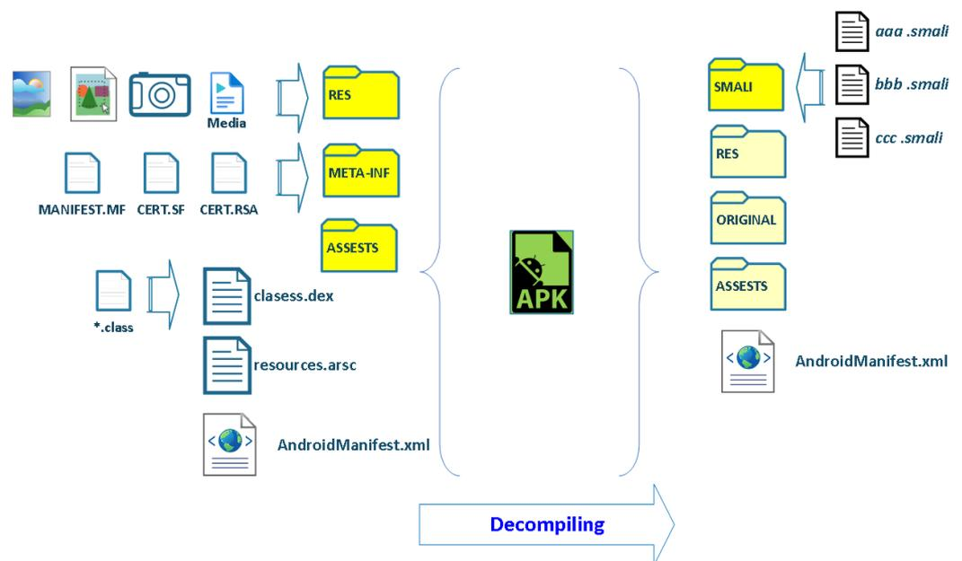
**Figure 1.** Android Application Package structure before and after the decompiling process. The diagram was generated based on the input and output generated by APKTool [8].
