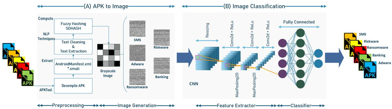
**Figure 3.** Proposed architecture: (A) APK to image conversion. This step transforms the APK into a grayscale image. (B) Grayscale images are analyzed in CNN for Android malware classification.
