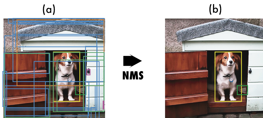
Figure 4. Non-maximum suppression (NMS). (a) Typical output of an object detection model containing multiple overlapping boxes. (b) Output after NMS.
