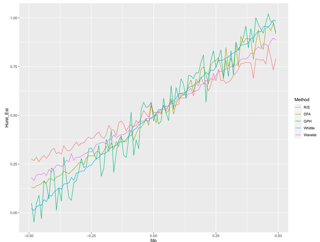
**Figure 8.** Comparison  $H$  vs.  $d$  of the estimation methods.
