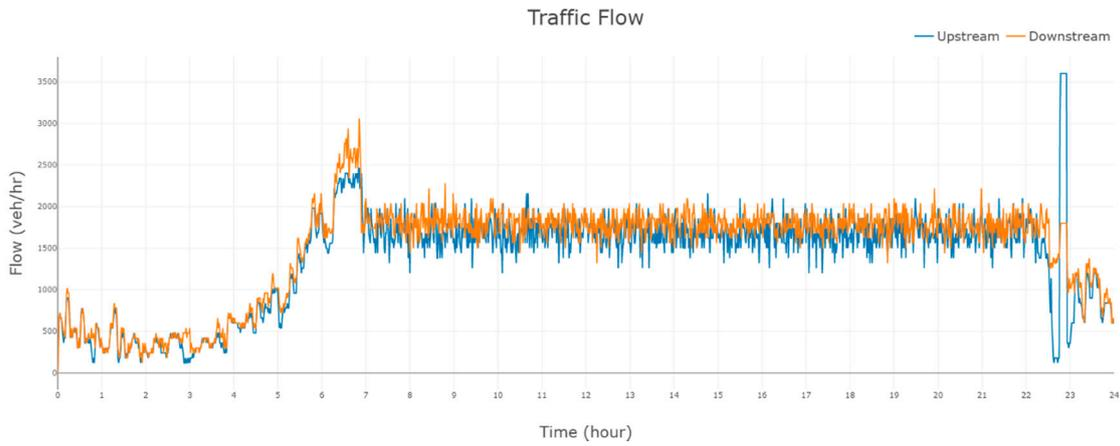
Figure 10. Traffic flow measured upstream and downstream of the ramp—no control scenario.
