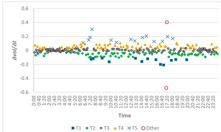
Figure 7. The five traffic types identified based on  $\Delta vol/\Delta t$ .
