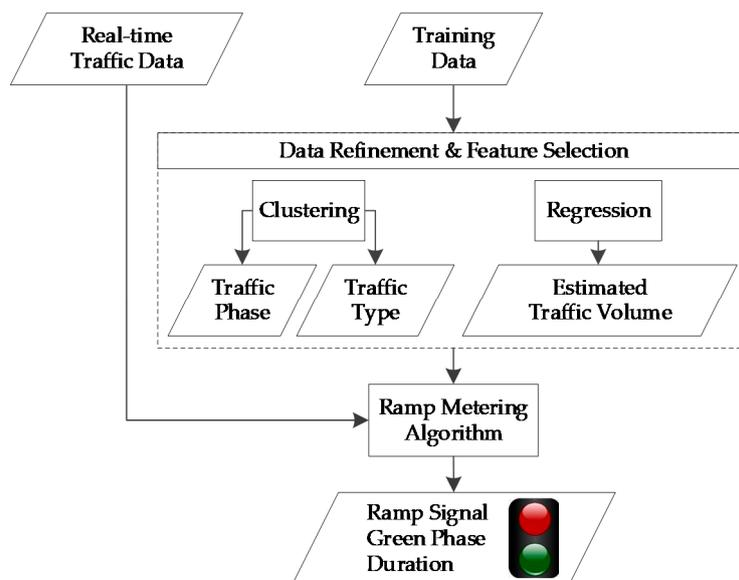
Figure 3. The general schema of proposed algorithm.
