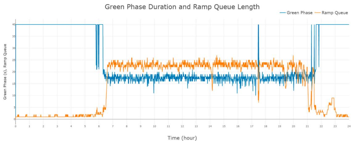
**Figure 18.** Green phase duration and ramp queue length—the proposed metering scenario.
