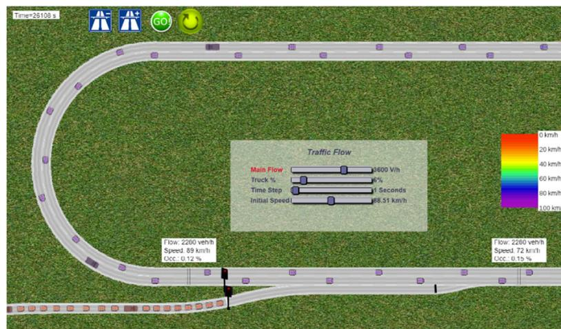
**Figure 9.** The ramp metering scenario simulated in MovSim.
