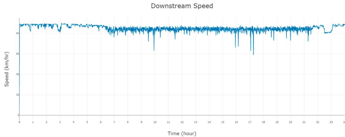
**Figure 17.** Average speed measured downstream of the ramp—the proposed metering scenario.
