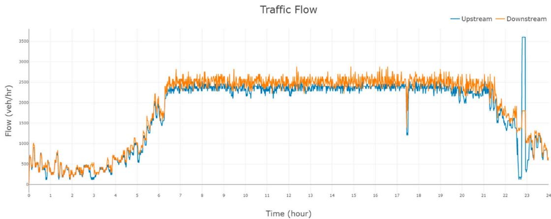
**Figure 16.** Traffic flow measured upstream and downstream of the ramp—the proposed metering scenario.
