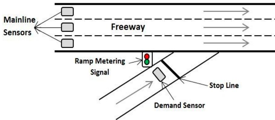
Figure 1. A typical ramp metering system.
