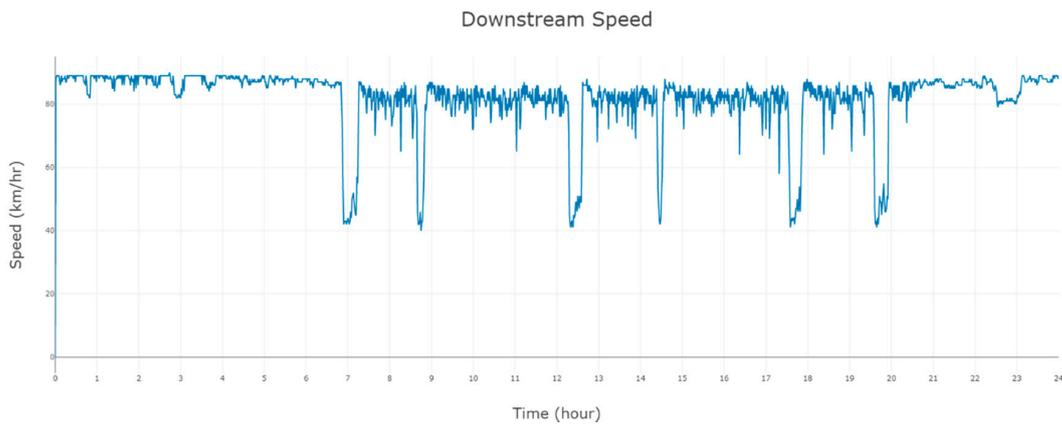
**Figure 14.** Average speed measured downstream of the ramp—ALINEA metering scenario.
