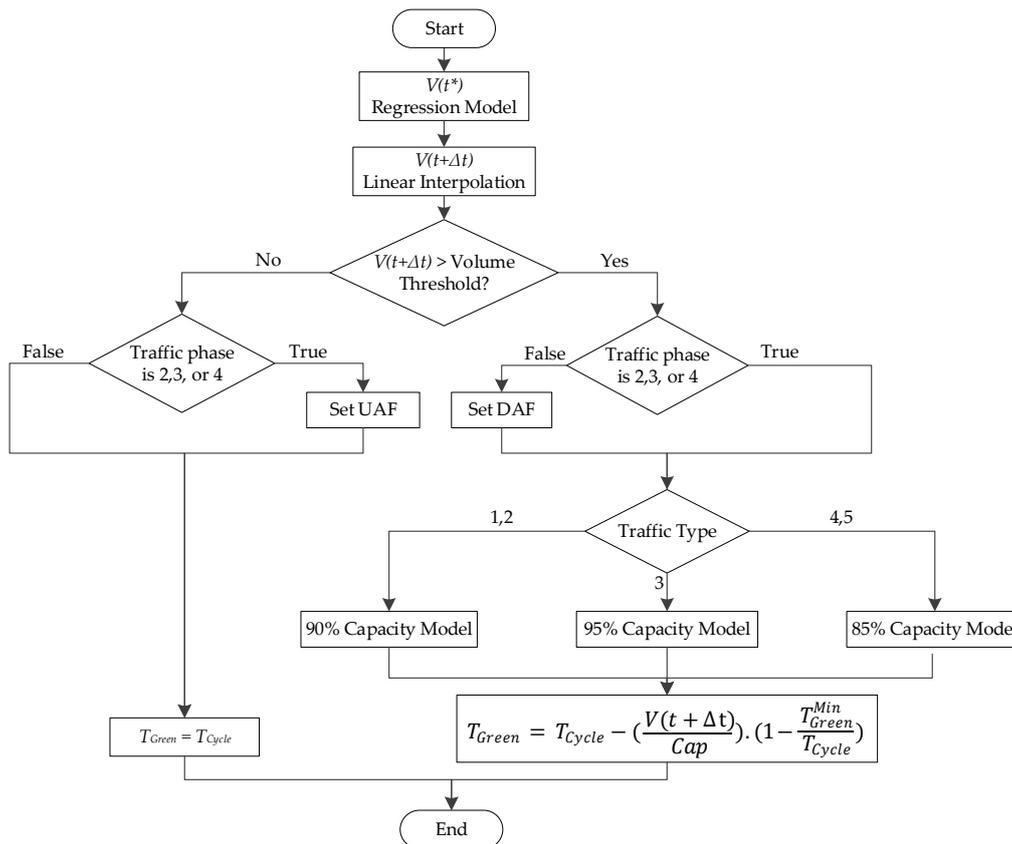
Figure 8. Proposed final ramp meter algorithm schematic.
