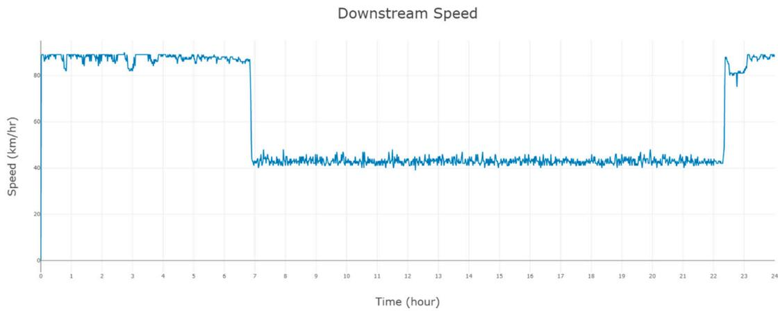
Figure 11. Average speed measured downstream of the ramp—no control scenario.
