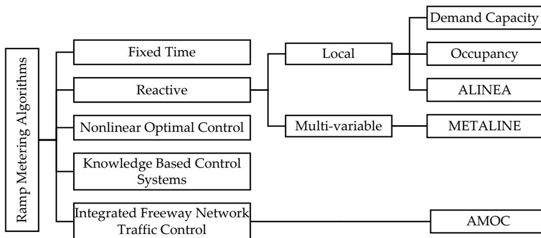
Figure 2. Ramp metering algorithms classification.
