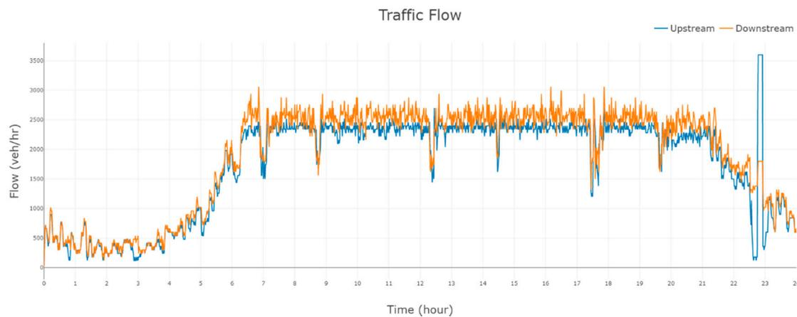
**Figure 13.** Traffic flow measured upstream and downstream of the ramp—ALINEA metering scenario.
