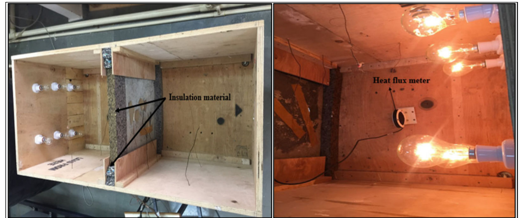
Figure 11. Wooden experimental setup by K. Sravani et al., reprinted with permission [222].
