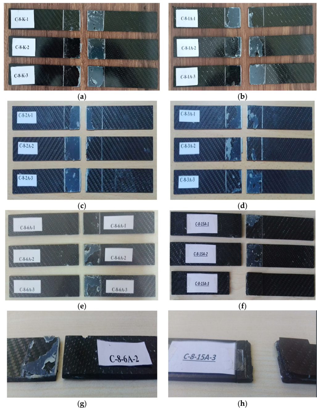
Figure 9. CFRP dry environment (a), 1st month (b), 2nd month (c), 3rd month (d), 6th month (e) and 15th month (f), adhesive bondline fracture (6th month) (g) and cohesive fracture (15th month) (h).
