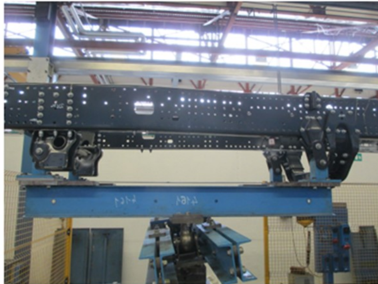
Figure 5. Front constraints of the HCV chassis frame.
