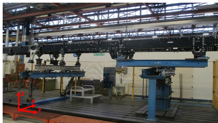
Figure 4. Test bench for an HCV chassis frame.
