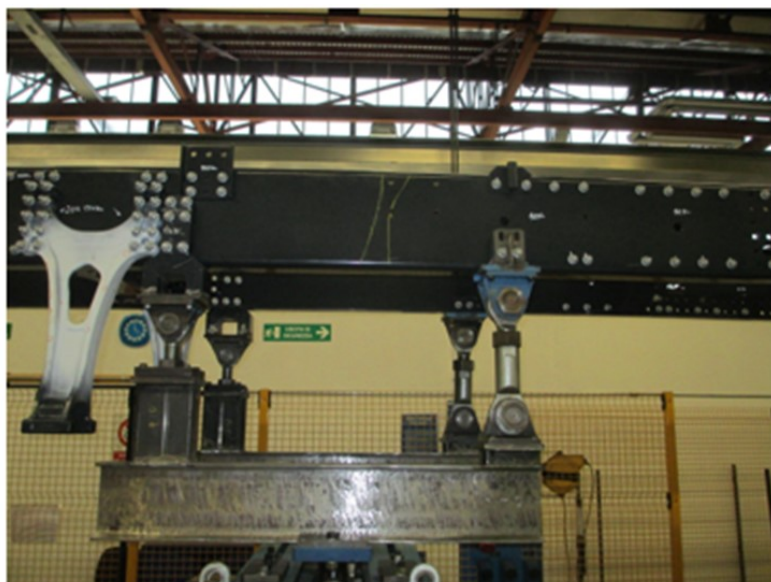
Figure 6. Rear constraints of the HCV chassis frame.
