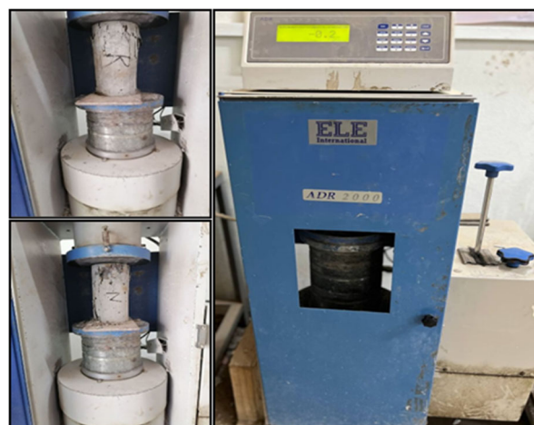
Figure 7. Compression strength testing.
