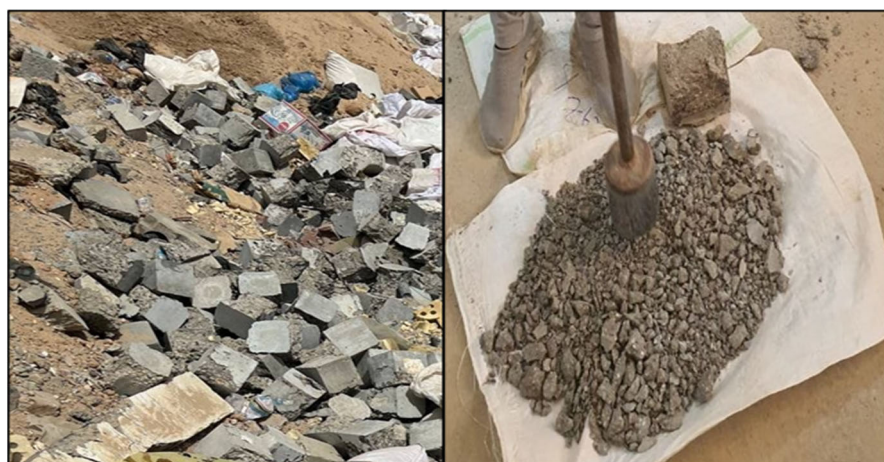
Figure 5. Assembly and crushing of waste concrete cubes.
