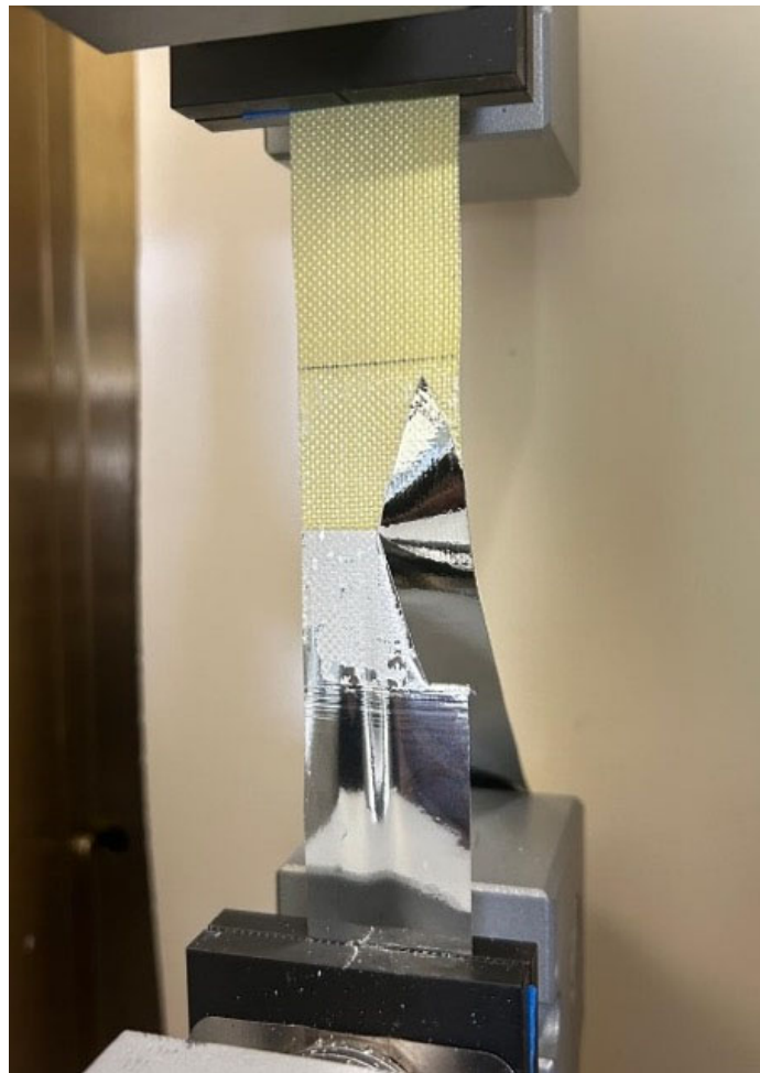
Figure 2. Film layer tearing during the T-peel test, affecting the adhesive strength measurement [7].
