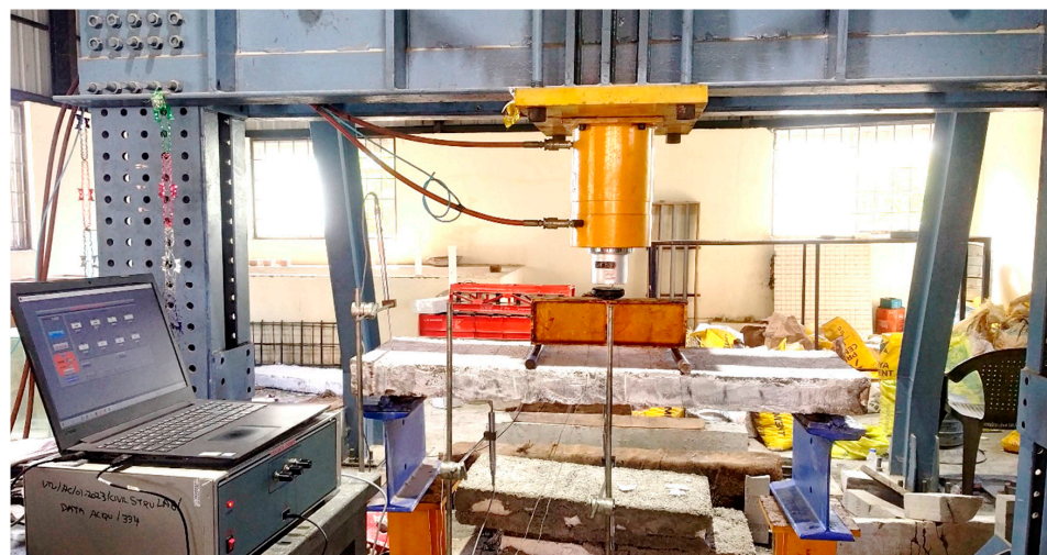
Figure 7. Loading arrangement with data acquisition system.
