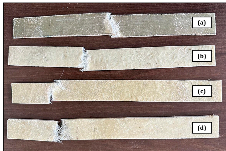
Figure 5. Tensile test specimens of (a) unfilled, (b) unhatched raw eggshell-filled, (c) unhatched boiled eggshell-filled, (d) post-hatched eggshell-filled composite variants.
