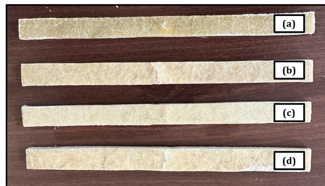
Figure 7. Flexural test specimens of (a) unfilled, (b) unhatched raw eggshell-filled, (c) unhatched boiled eggshell-filled, (d) post-hatched eggshell-filled composite variants.
