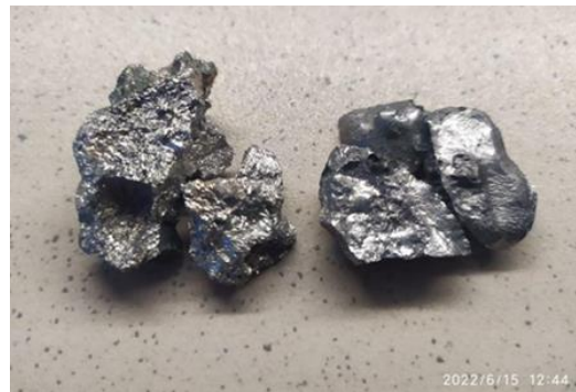
Figure 3. Alloy produced by melting at a temperature of 1800 °C.
