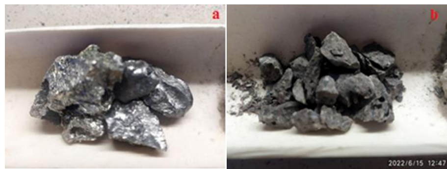
Figure 4. Alloy (a) and slag (b), produced by melting at a temperature of 1850 °C.
