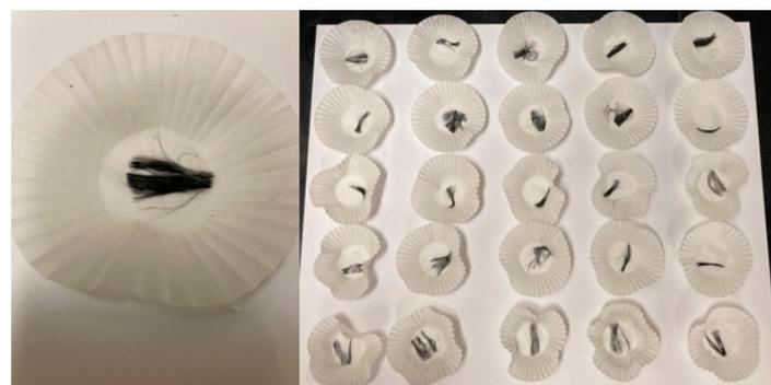
Figure 5. Solvent washed CFRP samples.
