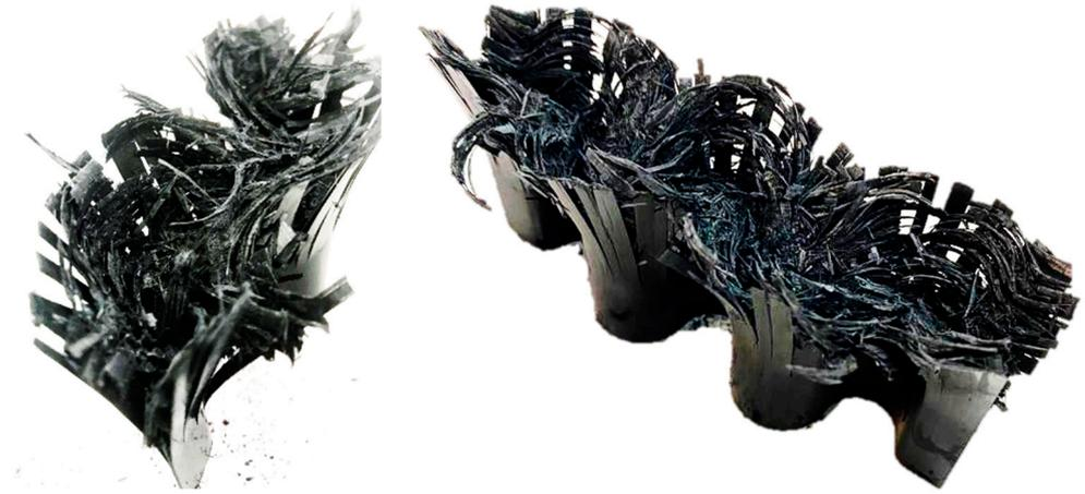
Figure 10. The deformed shapes of the sinusoidal specimens with 3 (left) and 5 curvatures (right).
