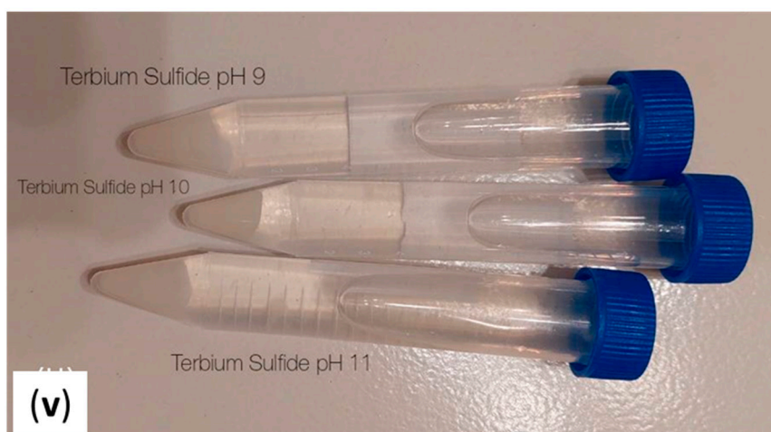
Figure S1. The process for preparing CS- \text{Tb}_2\text{S}_3 QDs by the wet-chemical method (steps i – v); whereas step (v) represents storage of the purified CS- \text{Tb}_2\text{S}_3 nanoparticles in ultrapure water.
