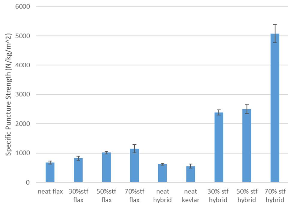
**Figure 7.** Comparison of specific puncture strengths.
