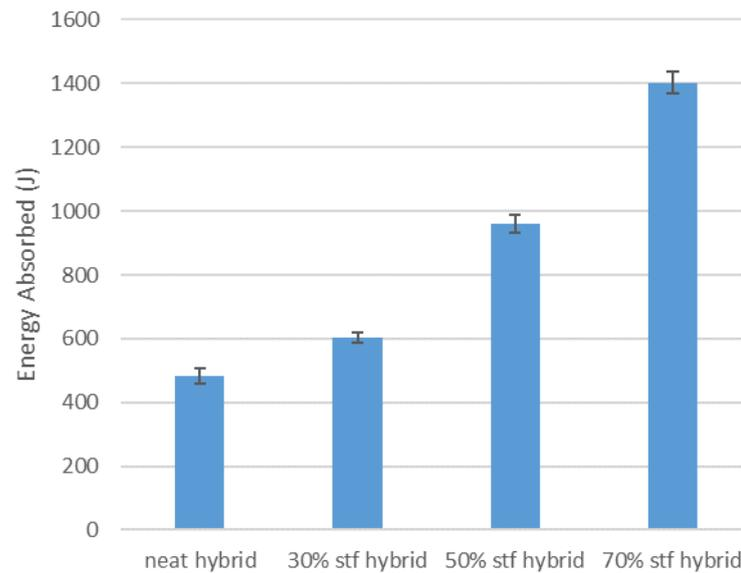
**Figure 10.** Comparison of ballistic impact energy absorption for hybrid samples.
