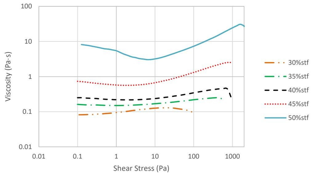
Figure 6. Effect of shear stress on viscosity at 50 °C.
