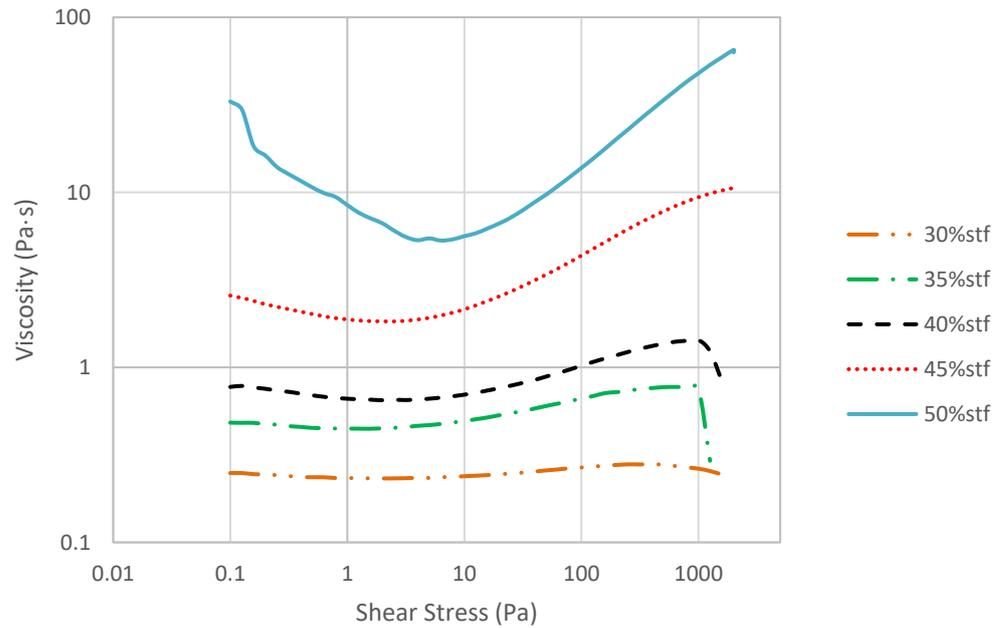
Figure 4. Shear stress effect on viscosity at 25 °C.
