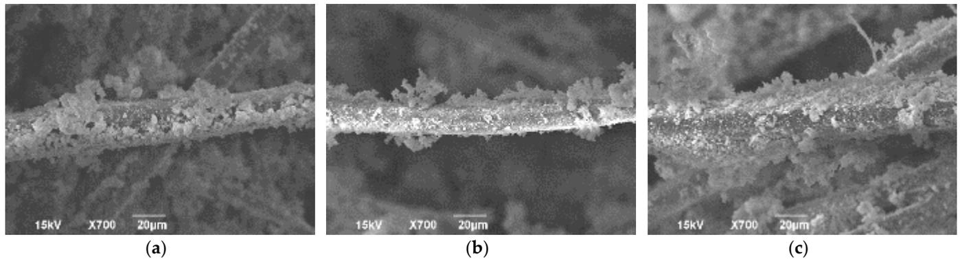
**Figure 13.** Nanosilica adherence to individual fibers. (a) 30% STF flax, (b) 50% STF flax, (c) 70% STF flax.
