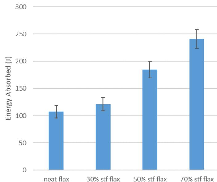
**Figure 9.** Comparison of ballistic impact energy absorption for flax fabric samples.
