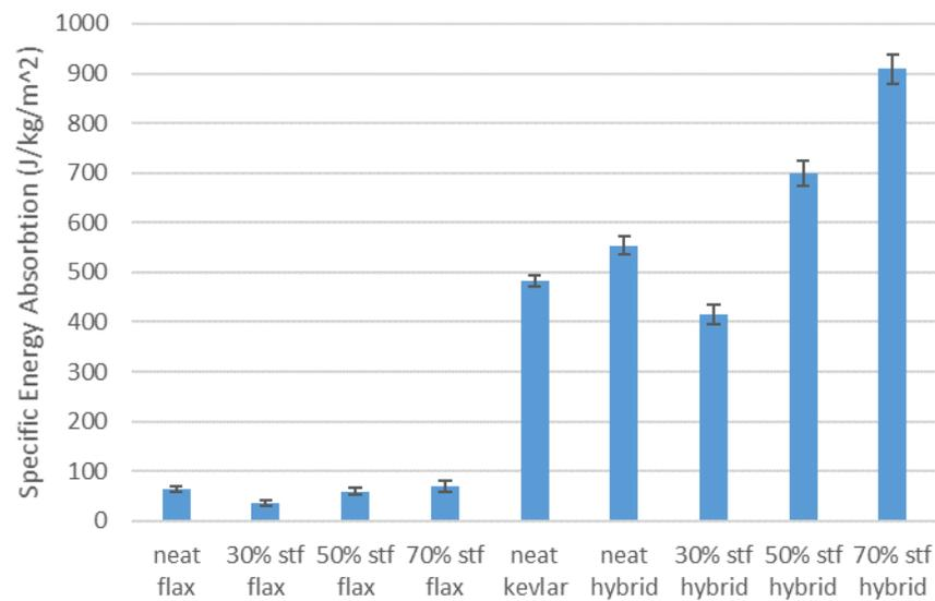
**Figure 11.** Comparison of specific ballistic impact energy absorption per layer.
