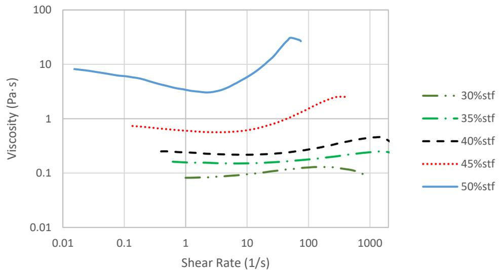
Figure 5. Effect of shear rate on viscosity at 50 °C.
