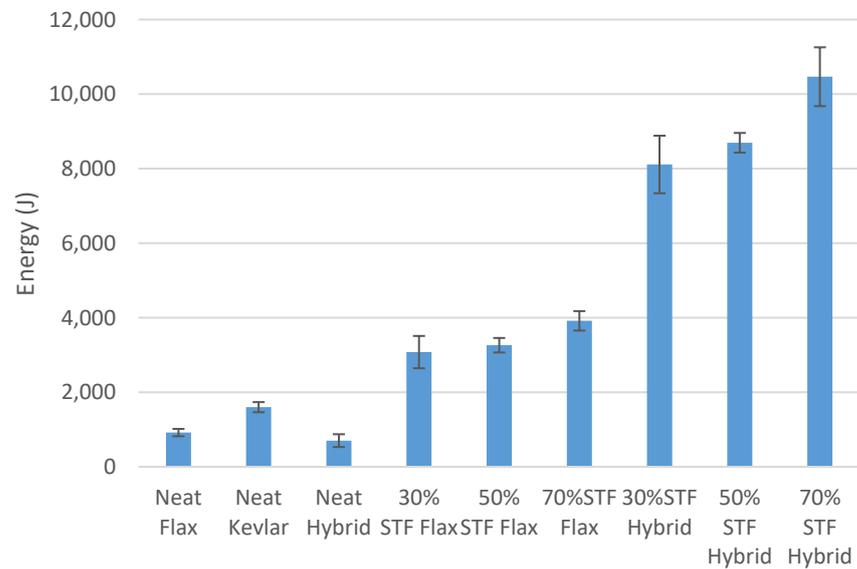
**Figure 8.** Comparison of average energy absorbed during puncture testing.
