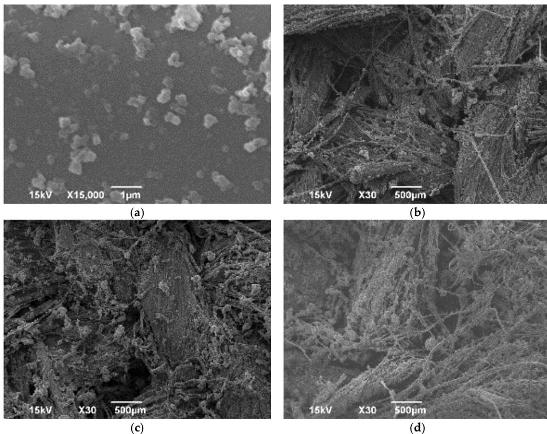
**Figure 12.** SEM images of (a) nanosilica particle agglomerates, (b) 30% STF flax, (c) 50% STF flax, (d) 70% STF flax.
