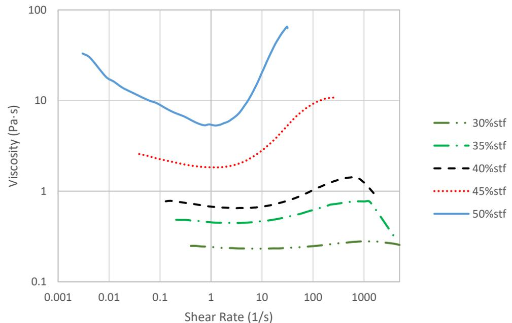
**Figure 3.** Shear rate effect on viscosity at 25 °C.
