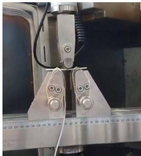
**Figure 2.** Three-point bending set up for cyclic loading of CFRP, GFRP, and hybrids.
