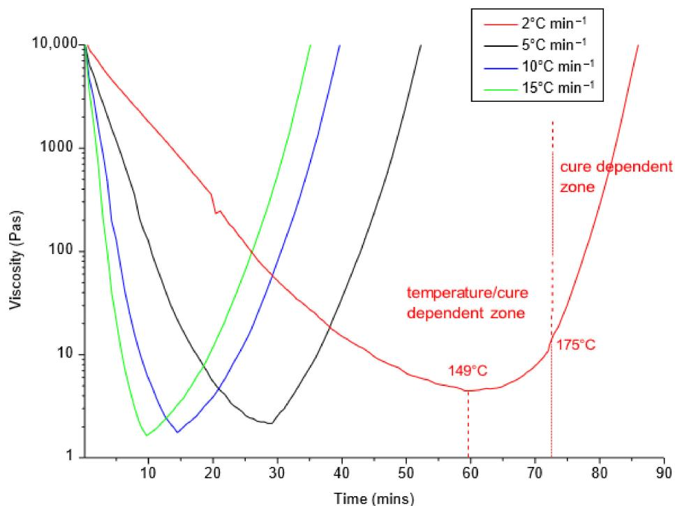
**Figure 12.** Resin viscosity as a function heating rates [99].
