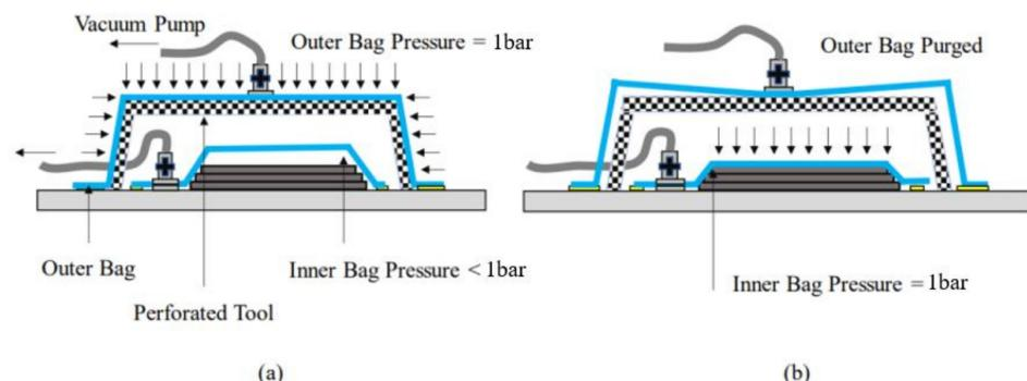
**Figure 3.** Schematics of a flexible double-vacuum-bagging setup with a perforated tool during (a) de-gassing phase and (b) compaction phase. Ref. [30] Reprinted with permission from Springer Nature.
