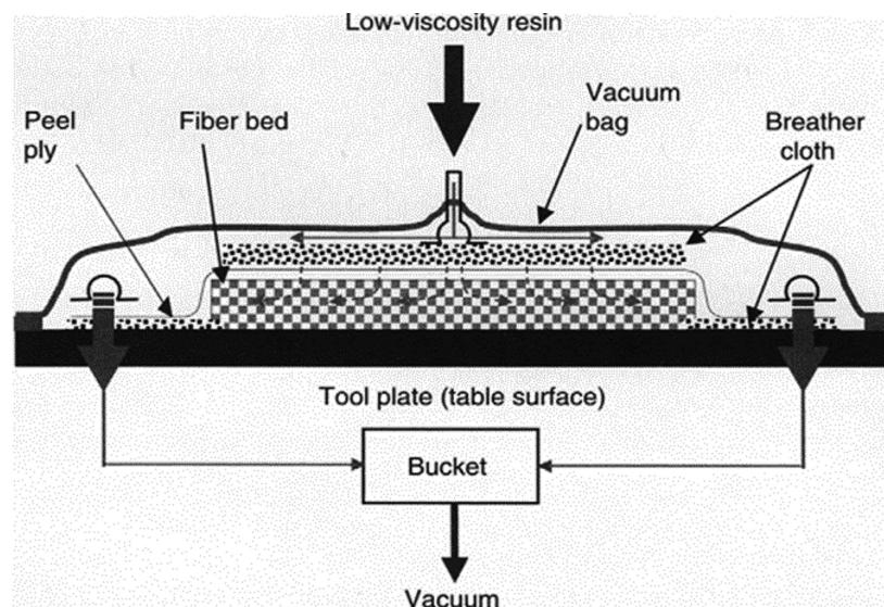
**Figure 8.** Schematics of VARTM [71]. Reprinted with permission from Elsevier.
