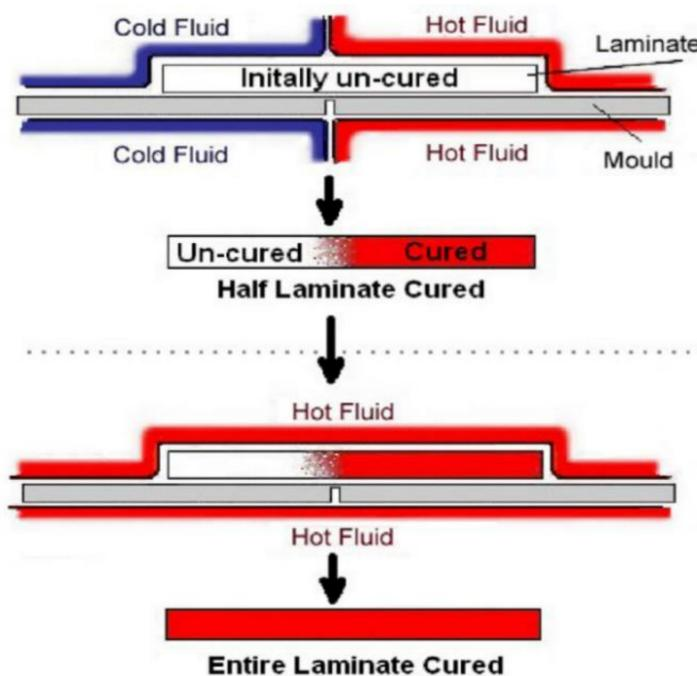
**Figure 11.** Schematics of the Melding Process [97]. Reprinted with permission from Elsevier.
