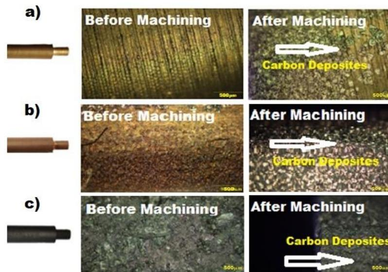
**Figure 31.** Microstructural changes of electrode material (a–c).
