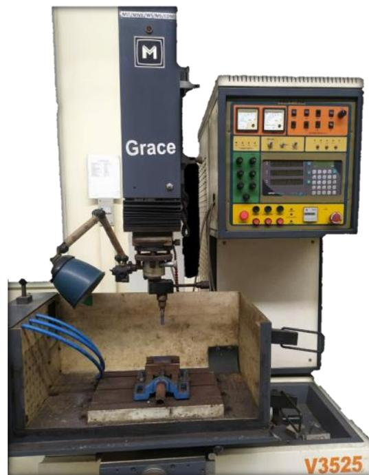
**Figure 8.** Electric discharge machining set up.
