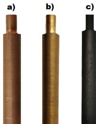
Figure 7. Electrodematerials: (a) brass, (b) copper, and (c) graphite.
