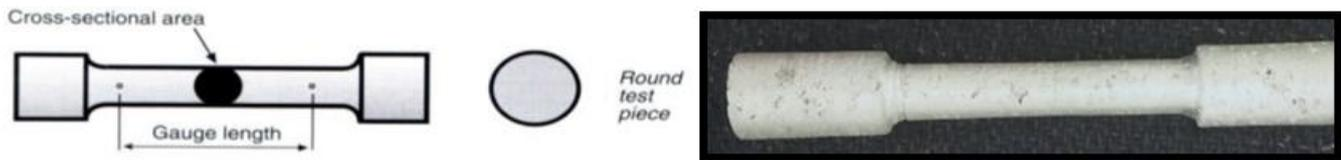
Figure 5. Tensile test samples.
