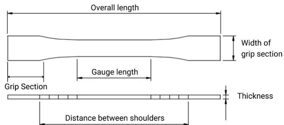
**Figure 2.** Schematic representation of tensile test specimen dimension as per ASTM D638-14 Standard.
