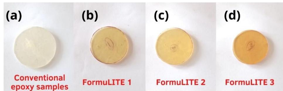
**Figure 6.** Water absorption test specimen dimension as per ASTM D570-98 standard, (a) conventional epoxy, (b) FormuLITE 1, (c) FormuLITE 2, and (d) FormuLITE 3.
