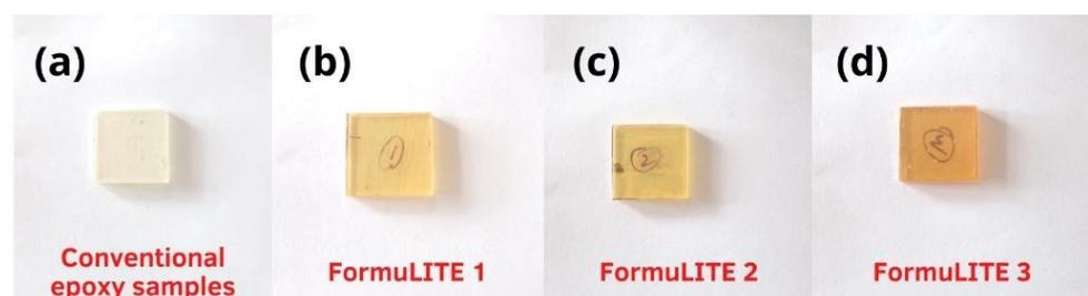
**Figure 5.** Hardness test specimen dimension as per ASTM E92-17 standard, (a) conventional epoxy, (b) FormuLITE 1, (c) FormuLITE 2, and (d) FormuLITE 3.
