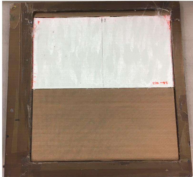
Figure 4. Sintered GFRP + powder epoxy half-plate inside steel frame.
