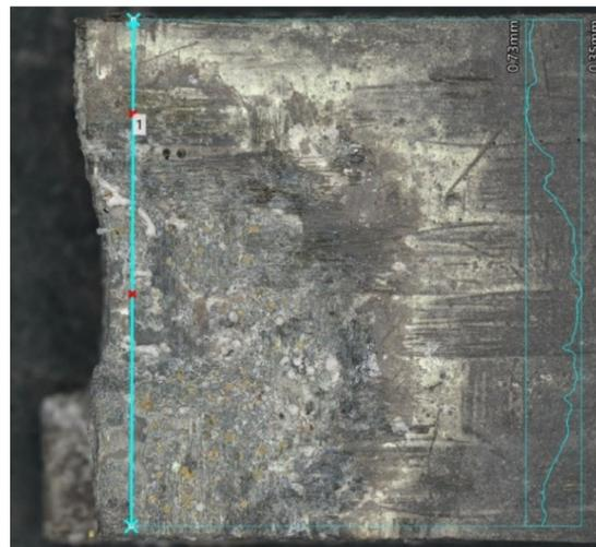
**Figure 13.** Optical image from a 3D optical microscope of face-view of fracture region of SA-MI specimen with depth profile across the width. The maximum depth ablated during high velocity exposure was about 0.38 mm.
