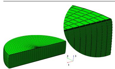
Figure 5. Meshed FREB model and detailed view.
