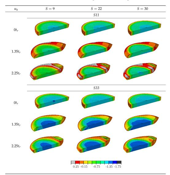
**Figure 8.** Influence of shape factor *S* on the axial normal stress *S11* and vertical normal stress *S33* distributions.
