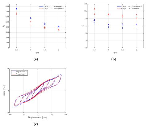
**Figure 7.** Comparison of predicted and experimental behaviors. (**a**) Experimental and predicted horizontal stiffness. (**b**) Experimental and predicted damping ratios. (**c**) Force-displacement curves under 4 MPa vertical pressure.
