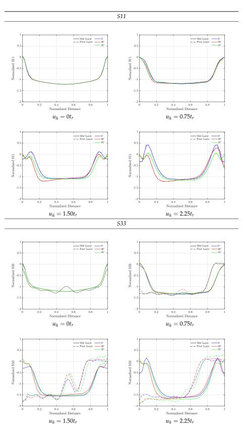
**Figure 20.** Normal axial *S11* and vertical *S33* stress along the symmetry axis. Effect of reinforcement orientation.
