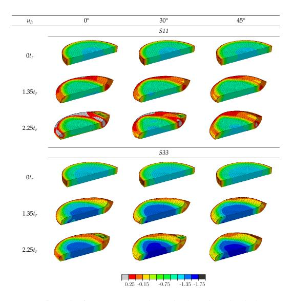
Figure 19. Influence of reinforcement orientation on the normal axial S11 and vertical S33 distributions.
