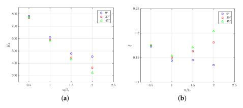
**Figure 23.** (a) Effective horizontal stiffness,  $k_h$ , and (b) equivalent damping ratio,  $\xi$ , under different reinforcement orientations.
