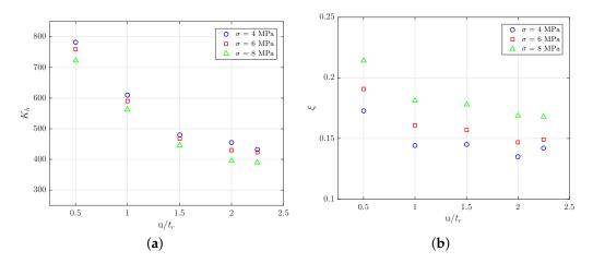
**Figure 28.** (a) Effective horizontal stiffness,  $k_h$ , and (b) equivalent damping ratio,  $\xi$ , under different compression levels.
