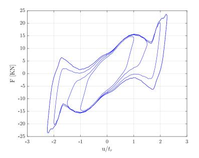
Figure 18. Force-displacement curve for 27RL\_22S.
