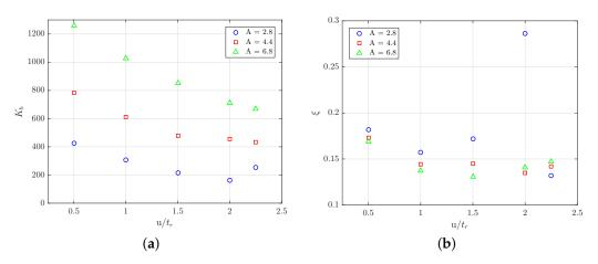
**Figure 17.** (a) Effective horizontal stiffness,  $k_h$ , and (b) equivalent damping ratio,  $\xi$ , under different compression levels.
