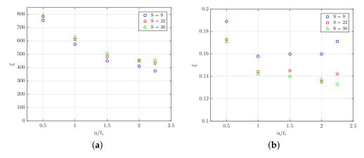
**Figure 12.** (a) Effective horizontal stiffness,  $k_h$ , and (b) equivalent damping ratio,  $\xi$ , under different values for the factor shape.
