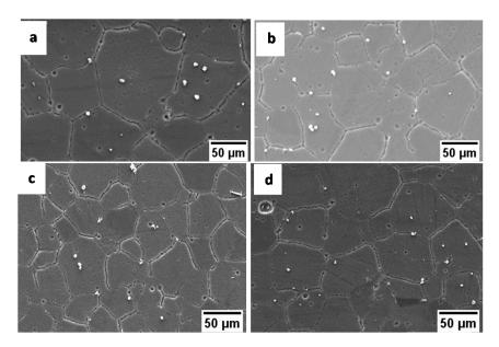
**Figure 4.** SEM images of aged AZ61 with CNTs: (**a**) 0 wt.%, (**b**) 0.1 wt.%, (**c**) 0.5 wt.%, and (**d**) and 1 wt.% [13].
