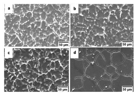
**Figure 3.** SEM images of as-cast AZ61 with CNTs: (**a**) 0 wt.%, (**b**) 0.1 wt.%, (**c**) 0.5 wt.%, and (**d**) and 1 wt.% [13].
