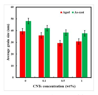
Figure 5. Average grain size AZ60/CNTs composites [13].
