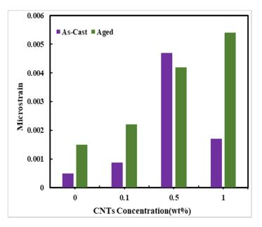
Figure 1. Microstrain distribution against carbon nanotubes (CNTs) concentration.
