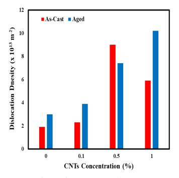
Figure 2. Dislocation density variation with CNTs concentration.
