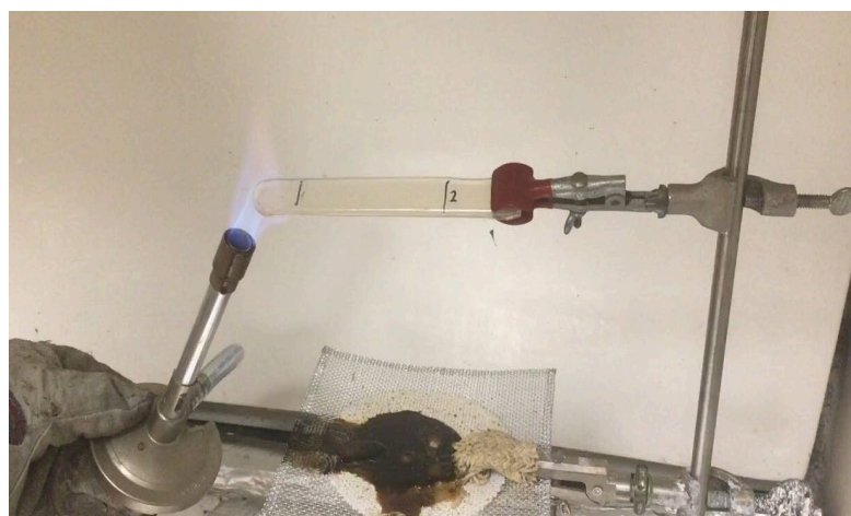
Figure 9. A picture showing the horizontal burn test (following ASTM D635–14 standard).
