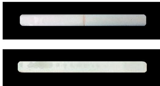
Figure 3. Notched samples before and after healing.
