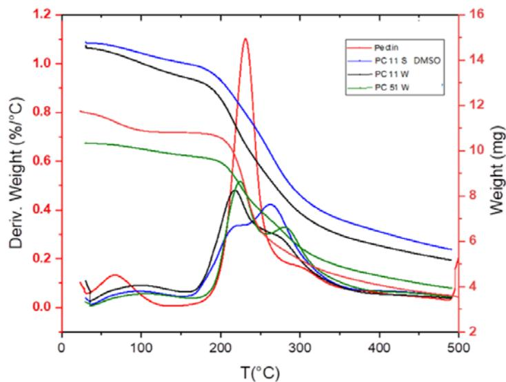
Figure 2. Thermal gravimetric analysis (TGA) results of pectin and pectin–chitosan composites.
