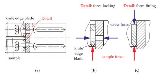
**Figure 2.** (a) Top view of the force-locking bearing attachment in loading (lateral) direction of a compression device according to Linke and García-Manrique [18], (b) forces in force-locking attachment (red: out-of-plane force of sample, blue: screw force), (c) forces in form-fitting bearing attachment (colours like before).
