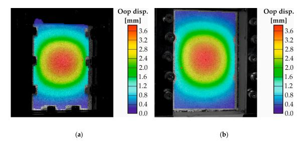
**Figure 12.** Out-of-plane displacement (Oop disp.) measured with DIC system illustrated on DIC camera picture of the (**a**) CAI device acc. to [18] (figure reproduced and adapted), (**b**) New CAI device with permission from [18].
