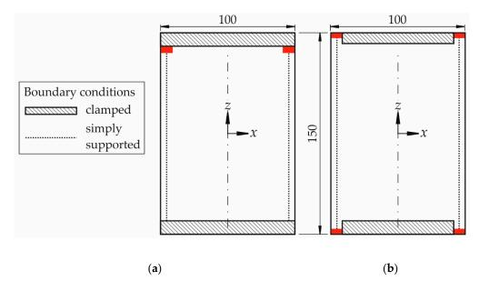
**Figure 3.** Schematic dimensions (100 by 150 mm<sup>2</sup>) of CAI sample and its supports (the unsupported areas are indicated in red) according to (**a**) EN 6038 [3], ISO 18352 [4] and SACMA SRM 2R-94 [5] and (**b**) AITM 1-0010 [2].
