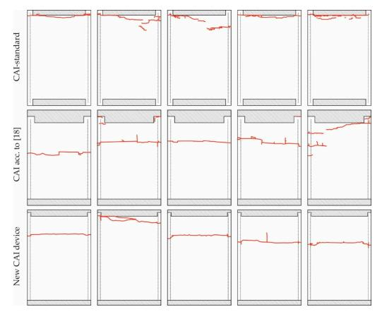
**Figure 9.** Fracture lines observable on sample surface for CAI-standard, modified CAI device (both results according to Linke and García-Manrique [18]) and proposed New CAI device (figure reproduced and adapted with permission from [18]).
