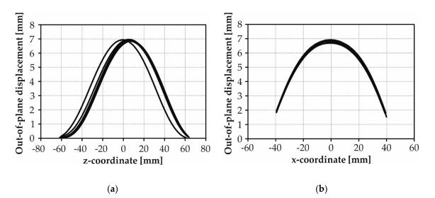
**Figure 11.** Out-of-plane displacements along the symmetrical line in the (**a**) global *z*-direction and (**b**) global *x*-direction of specimens tested with the New CAI device.
