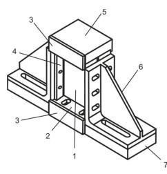
**Figure 1.** Schematically illustrated CAI test device and its components according to Flügge [19] with test plate (1), lower clamps (2), clamping plate (3), knife edge plates (4), top head clamping (5), angle frames (6) and base plate (7).
