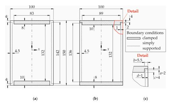
**Figure 6.** Boundary conditions for specimens according to (**a**) AITM 1-0010 [2], (**b**) new device, (**c**) geometric modifications of new device in CFRP design (figure reproduced and modified with permission from [18]).
