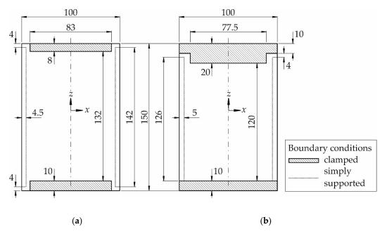
**Figure 4.** Boundary conditions for specimens (**a**) according to AITM 1-0010 [2] and (**b**) according to Linke and García-Manrique [18] (figure reproduced with permission from [18]).
