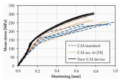
Figure 10. Mean stress versus shortening of specimens.
