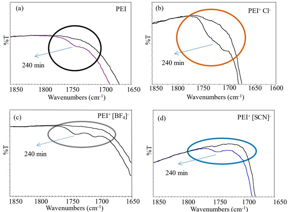
**Figure S4.** The FT-IR spectra between 1650-1850  $\text{cm}^{-1}$  wavenumber region of (a) bare PEI cryogel (b)  $\text{PEI}^+\text{Cl}^-$ , (c)  $\text{PEI}^+[\text{BF}_4]^-$ , and (d)  $\text{PEI}^+[\text{SCN}]^-$  PIL cryogels before and after 240 min  $\text{CO}_2$  exposure. [200 mL/min flow rate].
