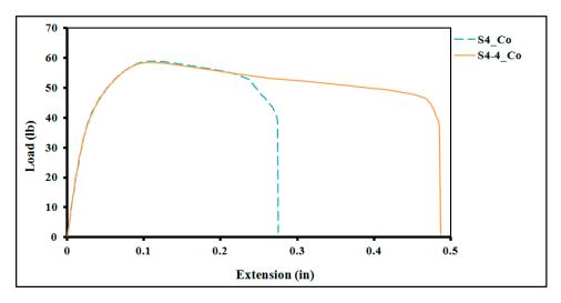
Figure 6. Load vs. extension curves of the S4\_Co and S4-4\_Co composites.
