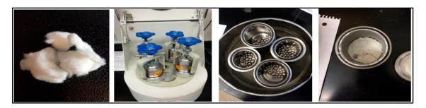
Figure 1. The cellulose pulp, ball mill, steel jars and balls, and powdered cellulose (left to right).
