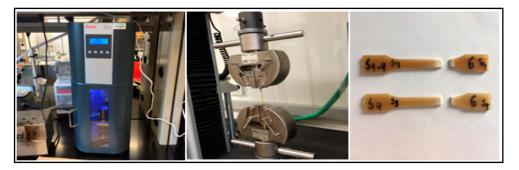
**Figure 2.** Injection molding and tensile testing machines, and the broken dog bone specimens after tensile testing (left to right).
