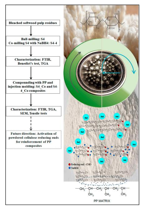
Scheme 1. Schematic illustration of the bull milling process.
