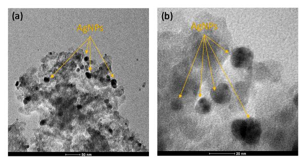
**Figure 2.** TEM images of Ag-loaded ZnO nanoparticles at different magnifications: (**a**) 43,000× and (**b**) 195,000×.
