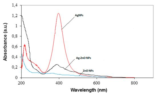
Figure 6. UV-Vis spectra of AgNP-decorated nano-ZnO particles (dispersed in water).
