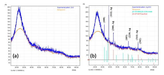
Figure 4. XRD patterns of (a) ZnO nanoparticles and (b) Ag/ZnO nanoparticles.
