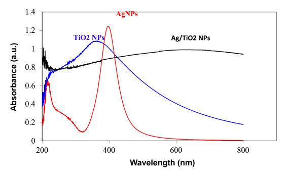
**Figure 5.** UV-Vis spectra of AgNPs, nano-TiO<sub>2</sub>, and AgNP-decorated nano-TiO<sub>2</sub> particles (dispersed in water).
