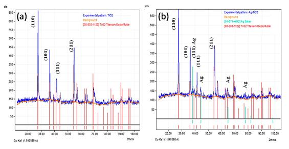
Figure 3. XRD patterns of (a) TiO<sub>2</sub> nanoparticles and (b) Ag/TiO<sub>2</sub> nanoparticles.
