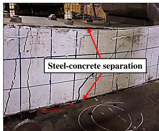
Figure 10. Steel–concrete separation in Rub-B specimen.
