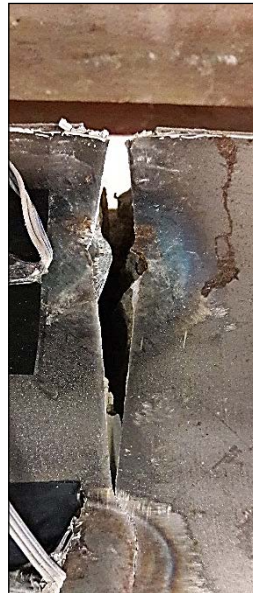
Figure 12. Steel rupture occurred at the bottom steel plate of the CC-W specimen.
