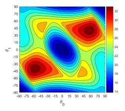
**Figure 5.** Critical temperatures for Graphite/Epoxy, SSSS variable-stiffness plates with lay-up  $[\pm \langle \theta_0 | \theta_1 \rangle_x]_s$ . Results obtained using ED3 theory.
