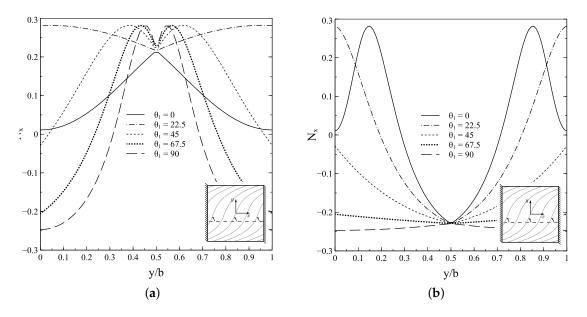
**Figure 7.** Pre-buckling membrane resultants for  $[\pm \langle \theta_0 | \theta_1 \rangle_y]_s$  laminates subjected to Case-Ty2 conditions: (a)  $\theta_0 = 15$ ; (b)  $\theta_0 = 75$ .
