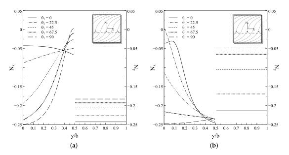
**Figure 6.** Pre-buckling membrane resultants for  $[\pm \langle \theta_0 | \theta_1 \rangle_y]_s$  laminates subjected to Case-Ty1 conditions: (a)  $\theta_0 = 15$ ; (b)  $\theta_0 = 75$ .
