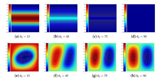
**Figure 9.** Pre-buckling and buckling results for SSSS variable-stiffness configurations, b/h = 50, and  $[\pm \langle \theta_0 | 90 \rangle_y]_s$ : (a)–(d): pre-buckling distribution of internal forces  $N_{xx}$ , (e)–(h): buckling mode.
