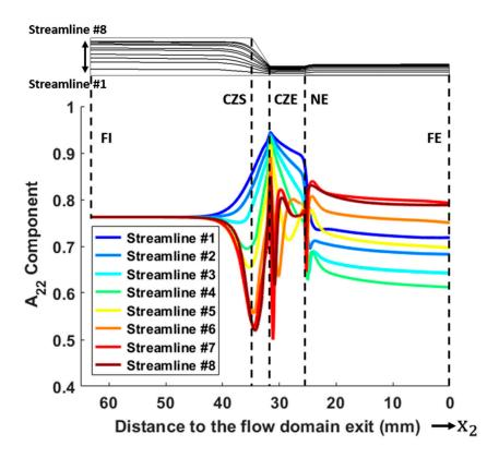
**Figure 9.**  $A_{22}$  component of fiber orientation solution computed using the flow kinematics solved by the PTT model at Q equates 100 mm<sup>3</sup>/s.
