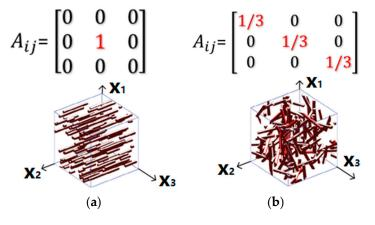
**Figure 7.** Fiber orientation tensors of (a) fully alignment along  $x_2$  direction and (b) uniformly random alignment.
