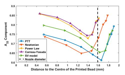
Figure 10. A<sub>22</sub> component at the flow domain exit solved using employed rheology models.
