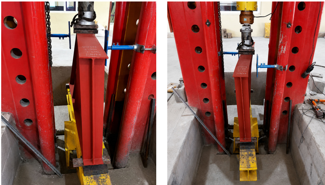
Figure 6. Specimen distortion during testing.
