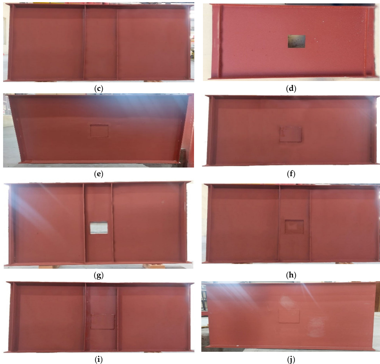
Figure 4. Images of specimen configurations. (a) BC beam control (no opening). (b) BC_NS beam control with no stiffeners at ends. (c) BC_TS beam control strengthening by two stiffeners at mid-span. (d) BO beam with opening of 180 \times 180 mm at mid-span. (e) BO_OP beam with opening of 180 \times 180 mm at mid-span retrofitted by one side patch plate. (f) BO_TP beam with opening of 180 \times 180 mm at mid-span retrofitted by two side patch plates. (g) BO_TS beam with opening of 180 \times 180 mm at mid-span retrofitted by two stiffeners. (h) BO_TS_OP beam with opening of 180 \times 180 mm at mid-span retrofitted by two stiffeners and one patch plate. (i) BO_TS_TP beam with opening of 180 \times 180 mm at mid-span retrofitted by two stiffeners and two patch plates. (j) BO_NS_TP beam with opening of 180 \times 180 mm at mid-span with no stiffeners at ends retrofitted by two side patch plates.
