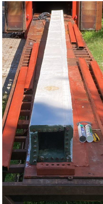
Figure 7. Full-scale steel-reinforced thermoplastic composite tower produced using the proposed manufacturing approach. The hollow-section geometry and integrated steel reinforcement demonstrate the applicability of the developed system at structural scale.
