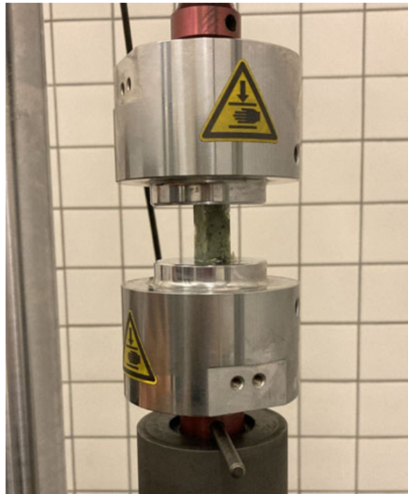
Figure 1. Compression test setup showing the prism specimen (12.7 mm × 12.7 mm × 25.4 mm) placed between the loading plates of the Instron testing machine.
