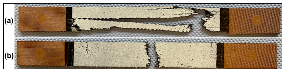
Figure 5. Fractured specimens from the quasi-static tensile tests: (a) Unidirectional material, (b) non-crimp fabric composite.
