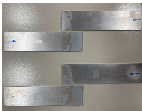
Figure 15. Examples of the “mixed” failure mode during the lap shear adhesion tests.
